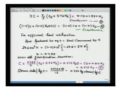
So, now, one can write down the chemical reactions as follows: so, I take x mole of Carbon plus x by 2 moles of O 2 plus 3.76 N 2; that is equal to x mole of CO plus 1.88 x into Nitrogen. Let me take this as my equation number 3. Then, I can write down 1 minus x moles Carbon plus 1 minus x H 2 O; let me consider vapor because we are supplying steam; that is equal to 1 minus x moles of Carbon monoxide plus 1 minus x moles of Hydrogen; this is my equation number 4.
