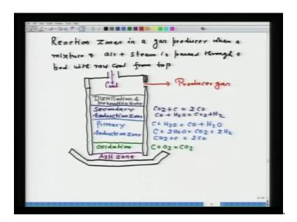
Now, let us consider reaction zones in a gas producer, when a mixture of air plus steam is passed through a bed, with raw coal from top. That means you have a reactor; coal is being fed; top up from top, bed is created and air steam is passing; so, it looks something like this (Refer Slide Time: 48:10).
