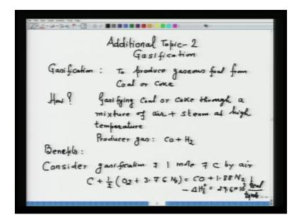
Now, gasification is in fact a unit process which is employed to produce gaseous fuel. So, gasification is a unit process which is used or which is employed to produce gaseous fuel from coal or coke because of obvious reason - because gaseous fuels are easy to handle. Mind you, the gaseous fuels that are produced by gasification are not classed as fossil fuel; they are the synthetically prepared fuel. The fossil fuel is natural gas which
