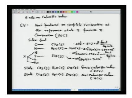
Now, before I proceed to calculation, I will like to make some note on calorific value because we will be doing some heat balance. So, a note on calorific value: It is important to know what calorific value is - a note on calorific value and the listeners of this video, for the details, one can see the video lectures on fuel furnace and refectory where, a calorific value is dealt with in detail over there. Here, I will be presenting whatever is important.
