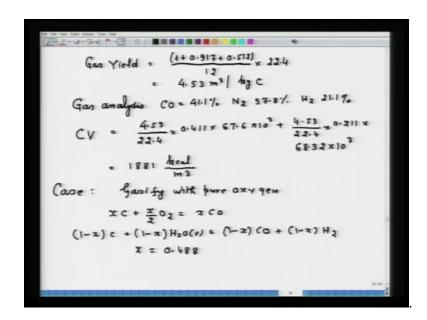
You can also calculate, gas yield. You can also calculate; that means, how much amount of gas is produced per kg or kg mole of Carbon, whichever way? So, that is, straightaway one can put it say 1 plus 0.917 plus 0.512; that is the right hand side of the equation 5. If we divided by 12, and of course, you have to multiply by 22.4; so, the gas yield would be equal to 4.53 meter cube per kg Carbon.
