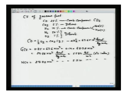
Now, similarly, an example can be given. So, one wants to calculate calorific value of gaseous fuel; CV stands for calorific value; CV of gaseous fuel, the definition remains same - gross or net calorific value. Now, suppose, let us say CO is equal to 25 percent, CO 2 let us take 5 percent, Hydrogen let us take 19 percent, Nitrogen let us take 50 percent and Oxygen let us take 1 percent.
