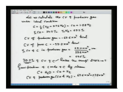
Now, let us calculate the calorific value of a producer gas under ideal condition. So, let us calculate the calorific value of producer gas under ideal condition, by ideal conditions; I mean, you are gasifying pure Carbon with air.
