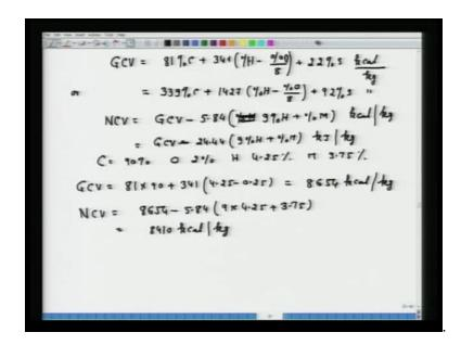
We all know this value if we convert these values on kg basis, If we take 1 kg of the fuel and we try to calculate, then we can calculate gross calorific value, that is equal to 81 into percent Carbon plus 341 percent H minus percent O upon 8 plus 22 into percent Sulphur and its unit is kilocalorie per kg.
