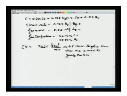
Now, as regards the heat balance, you have to make the heat balance; you can calculate the value of x and that will come up to be same as we calculated earlier - 0.488 as calculated previously. So, our equation would be C plus 0.244 O 2 plus 0.512 H 2 O; that will be equal to CO plus 0.512 H 2 .
