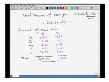
So, first I will write in kg moles. So, Carbon monoxide is 1.1268, CO 2 1.7966, and Nitrogen 8.7232 and in percent, this becomes 9.67, 15.43 and 74.90. Now, we can calculate total amount of exit gas; of course, we have to sum total and that will be equal to 11.6466 kg moles per minute and this becomes equal to 260.88 meter cube per minute.
