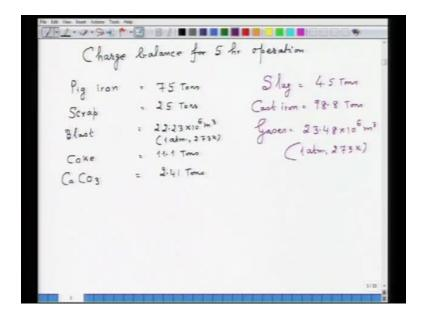
Now, it is also being asked, what is the charge balance for 5 hour operations? So, I am making now charge balance for 5 hour operation. That means, if suppose the cupola operates for 5 hours, how much charge we have to keep in reserve? So, this can be calculated. So, we will be needing pig Iron; that we will require 75 tons, scrap 25 tons.
