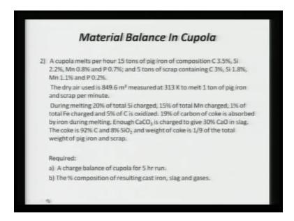
Now, here is the second problem and second problem says a cupola melts per hour 15 tons of pig Iron of composition: Carbon 3.5 percent, Silicon 2.2 percent, Manganese and phosphorus composition is given. 5 tons of scrap containing this; this is the composition of a scrap. Now, note - as I said in the burden, pig Iron plus coke plus scrap and Calcium Carbonate.
