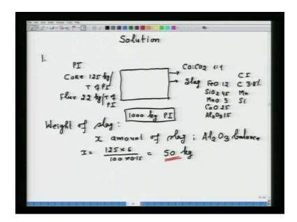
Let us take the solutions. Problem number 1 and let me represent the problem as a block diagram. So, as an input, we have pig Iron and then coke; coke amount is 125 kg per ton of pig Iron and flux we are having 22 kg again, per ton of pig Iron.
