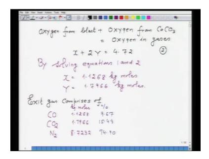
Now similarly, we have to do the oxygen balance. So, I am performing oxygen balance and this oxygen balance is oxygen from blast plus oxygen from Calcium Carbonate that is equal to oxygen in gases. Now, I will just write down in terms of the equation. So, the equation becomes x plus 2Y that is equal to 4.72 and this is our equation number 2.
