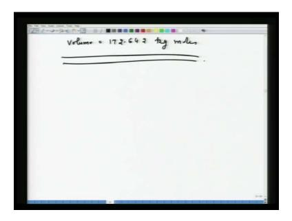
The last thing, which is left is, the volume and percentage composition of blast furnace gas. In order to calculate the volume of gas, we have already calculated CO CO 2. All that we have to calculate is nitrogen. So, if you do... We have to add H 2 O. So, volume of gas will be equal to 172.642 kg moles. That makes the calculation of charge balance complete.
