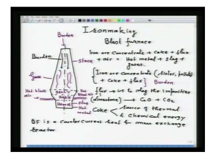
Now, as all of you know, the reactor in which iron is made is called blast furnace. So, as such this is the blast furnace iron making. On my left, this is the sketch, which I have
