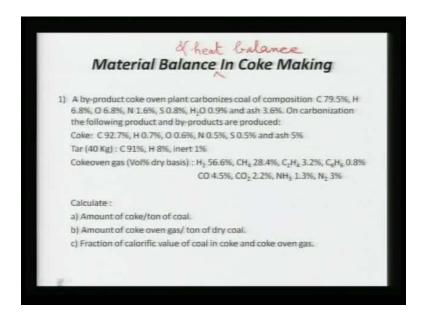
Typically, in the coke making industry, a byproduct coke oven is used to produce coke from coal and all of you know that coal is heated out of contact of air. You can also call this process as carbonization.
