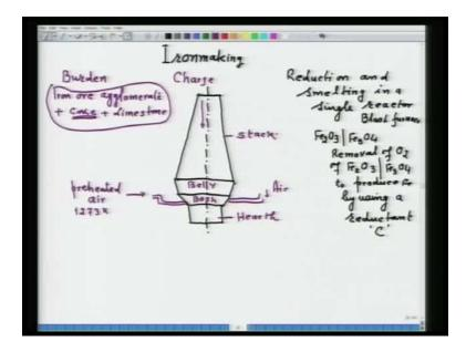
Now, the sketch, which I have drawn, is a blast furnace and it is used for ironmaking. Before I describe the sketch, I would like to say that the blast furnace ironmaking typically implies a reduction and smelting in a single reactor. The sketch before you is called a blast furnace and I hope all of you must be aware of it.
