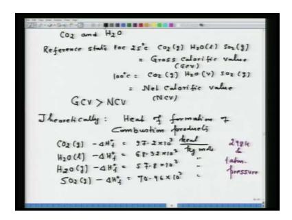
Now, if you see the composition, it has carbon, hydrogen, oxygen, nitrogen and sulphur is very minimum. So, the combustible components are carbon and hydrogen, CO2 and H2O are mainly the products of complete combustion of the coke. For example, let us take the reference state, if we take Poc reference state at 25 degree celsius, then CO2 is in the gaseous state, H2O as liquid and SO2 in the gaseous state. What do we determine? We have gross calorific value.
