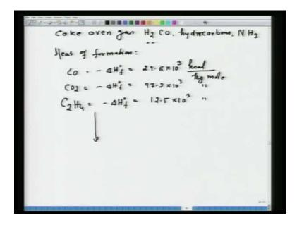
Now, think of the coke oven gas. Coke oven gas contains hydrogen, carbon monoxide, hydrocarbons, it may contain NH3 and these are all combustible components. So, in order to find out the calorific value of coke oven gas... We can also find out the calorific value of coke oven gas by the heat of formation value. So, I am giving heat of formation, for example, CO is minus delta H naught f equal to 29.6 into 10 to the power 3 kilocalorie per kg mole.
