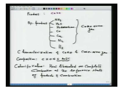
When coal is destructively distilled or coal is carbonized, we get the product and byproducts. I will be writing only the product because my objective of using coal and coke oven is to produce coke and so the product is only coke. Whereas, the byproducts could be NH3, H2S, hydrocarbons like C2H4, CO2, nitrogen and all these are called coke oven gases.
