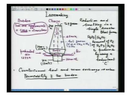
So, the hot gasses comprises of CO plus CO2 plus N2 plus H2O. They travel upward that means this blast furnace is essentially a counter current heat and mass exchange reactor. These are some of the important thing that we must know: first thing that a blast furnace is a counter current heat and mass exchange reactor. In this counter current, the heat and mass are exchange is between the burdens or between the descending burdens with the ascending gasses.
