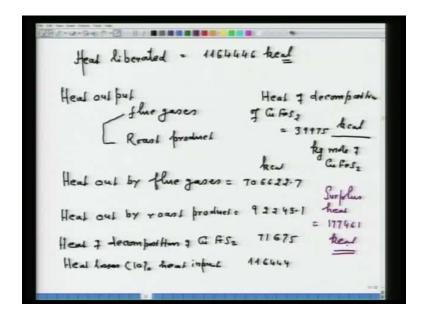
Here, the chalcopyrite concentrate consist of Cu Fe S 2. So, one is to have some heat of decomposition of Cu Fe S 2 that also we have to consider.
