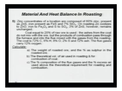
Now, problem fifth; again, it is roasting of zinc concentrate, but here you are using coal; coal composition is given. Here, both the products of combustion as well as the roasting gases which are evolved, both are mixed and they are going to be together. There are little bit different in the statement of the problem, the solution may not be similar to the earlier, but there is a little bit difference and you have to catch that particular point to solve that problem.
