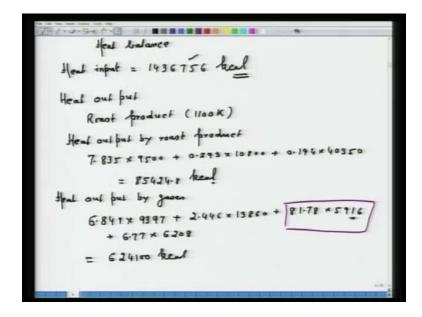
So, for the quick estimation I am writing here 6.849 into 9397 plus 2.446 into 13860; that is h 1100 minus h 298 for SO 3 plus 81.78 into 5916; 5916 is the h 1100 minus h 298 for nitrogen and plus 6.77 into 6208. So, total heat carried away by the gases that will be 624100.
