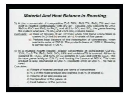
So, the problem 3 refers to the roasting of zinc concentrate. The compositions are given, the conditions are given and the roast product which came for under the given conditions of roasting is given. You have to find out rate of blowing air, excess air and analysis of flue gases. I have
