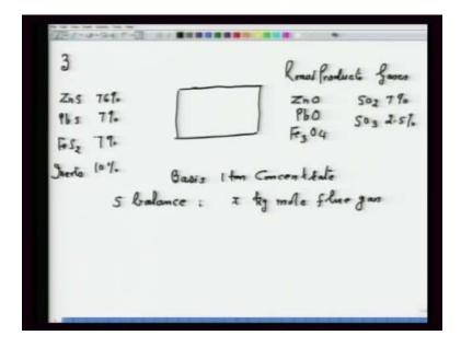
So, by doing that sulphur balances you can calculate the amount of flue gas. So, as such I am performing sulphur balance - I am performing sulphur balance.
