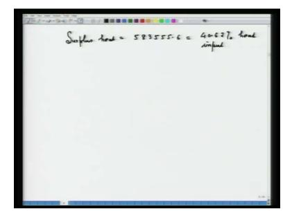
If we do that then the losses will be 143675.6, so total heats out that will be 853200.4. So, roasting of zinc concentrate in this particular problem, it is unaccompanied by a surplus heat and this surplus heat is 583555.6 that constitute around 40.62 percent of heat input.
