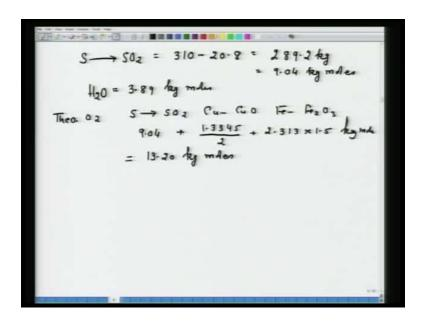
You can take it for granted that sulphur is converted according to stoichiometry of the reaction and SO 2. So that makes your life little easy. We have to now calculate theoretical oxygen and theoretical oxygen that will be S to SO 2, Cu to Cu O and Fe to Fe 2 O 3. This is where you will be requiring oxygen, so you can calculate the oxygen S to SO 2 that will be 9.04 plus Cu to C O 1.3345 upon 2 plus 2.313 into 1.5. Mind you they are all in kg moles.
