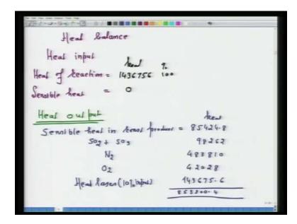
Now, if you do the heat balance, just to illustrate what I have written or said, so heat input that will be the heat of reaction and nothing else. That is equal to 1436756 in kilocalorie; that means, 100 percent of the heat which is required for the roasting is supplied by the heat of reaction that is what the 100 percent means.
