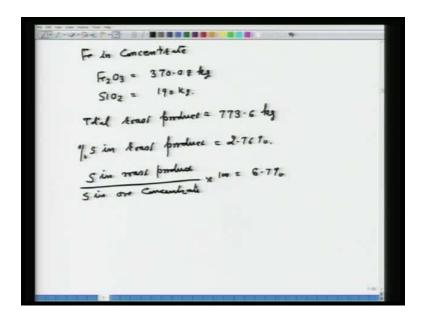
You have to calculate the Fe 2 O 3, so you calculate iron in the concentrate and then you calculate Fe 2 O 3 from that. So, Fe 2 O 3 would be 370.08 kg; this you can calculate. Of course,
