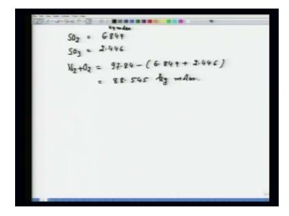
So, N 2 plus O 2 that will be equal to 97.84 that is amount of flue gas minus 6.849 plus 2.446, so that makes 88.545; mind you all in kg moles. What to do now? We have to know nitrogen and oxygen. Now here, you have to make use of that the kg mole of air, 1 kg mole oxygen, 3.76 mole of nitrogen.
