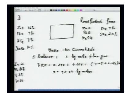
Now, I can straight away solve this equation. So, the flue gas that will be coming is 97.84 kg moles. Now, I know the amount of flue gas. However, you can also like to do it; you can also take sulphur balance x kg or x meter cube flue gas. Accordingly, you can also calculate, the choice is yours, the way you want to proceed.
