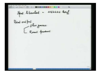
Heat liberated, I will be straight away multiplying the moles with the values of the heat of formation of the product. So, if I do that then heat liberated will become 1164446 kilo calorie that is the thing. Now, heat output; one heat output will be as usual by flue gases and another heat output will be roast product.
