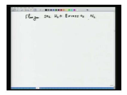
The flue gas will contain what SO 2, H 2 O, then excess oxygen and nitrogen. Now, nitrogen I can divide in two parts according to my problem one, corresponding to the theoretical and another corresponding to excess oxygen, there will be excess nitrogen also.
