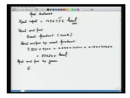
Heat output by roast product - or if you wish, I can just write down some of the value, so that will be 7.835 into 9500 plus 0.293 into 10800 plus 0.194 into 40350. Now, you have to sum total, so heat output will be equal to 85424.8 kilo calorie. Similarly, you have to calculate heat output by gases or heat carried away by gases, whichever way you want to understand. You know all the gases SO 2, SO 3, N 2 and oxygen.
