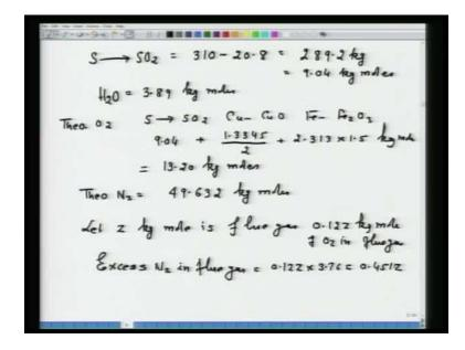
So, you have to do now, let z kg mole is the flue gas. So, 0.12 z kg mole of oxygen in flue gas, you agree with me? Now, what to do? I know now, the excess oxygen in the flue gas is 0.12 z, so accordingly excess nitrogen, how much it will be? Excess nitrogen in flue gas that will be equal to 0.12 z into 3.76 that will be equal to 0.451 z.
