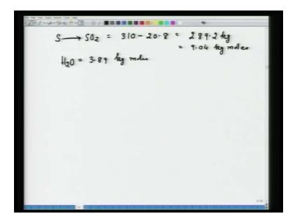
So that means, since we know this sulphur which is in the roast product, so I can calculate sulphur which is going to SO 2 that will be equal to 310 minus 20.8 that will be equal to 289.2
