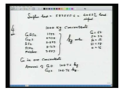
First, let us find out the copper in ore concentrate that you can find out, divide into 50 percent. So then, you can calculate amount of Cu O and amount of Cu 2 S, now both these amounts are coming 106.76 kg and this amount is also 106.76 kg.
