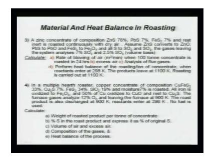
Again, you have to calculate here the percentage of sulphur in the roast product, weight of roast product, volume of air and also I have given you, you required to calculate heat balance process.
