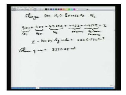
So, it is very easy now, I can write down on 9.04 plus 3.89 plus 49.632 plus 0.12 z plus 0.451 z that is equal to z. Now, this is SO 2, this is H 2 O, this is theoretical nitrogen, this is excess oxygen and this is nitrogen corresponding to excess nitrogen corresponding to excess oxygen that is all (Refer Slide Time: 40:17).
