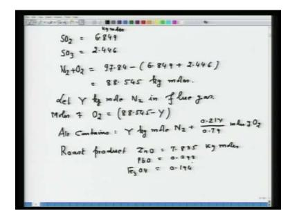
Now, let us consider Y kg mole is nitrogen in flue gas. Then, how much will be oxygen? Oxygen will be equal to 88.545 minus Y that will be moles of oxygen. What air contains? Air will contain Y kg mole nitrogen plus 0.21 Y upon 0.79 moles of oxygen. After this, we have to also we have to find out the analysis of roast product. So, the roast product as per the statement of the problem it consist of Zn O that will be equal to 7.835 all in kg moles, Pb O 0.293 and Fe 3 O 4 that is equal to 0.194.
