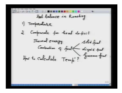
The first information that we would like to have is the temperature attainted by the roast product inside the reactor. Why this temperature is important? This temperature is important because you have to find out the material for the construction of the reactor. Now, material must be able to sustain that particular high temperature. It means that material should not fuse at that temperature.
