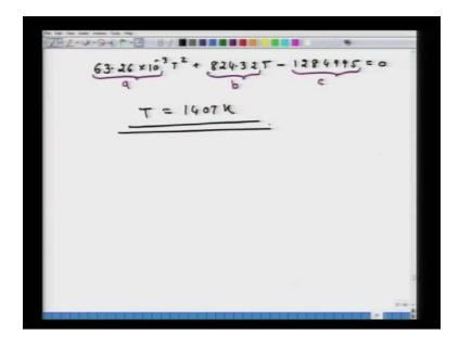
So, I am arranging the equation in a quadratic form. It will be 63.26 into 10 to the power minus 3 T square plus 824.32 T minus 1284995 and that is equal to 0. You know that the value of this is a, this is the value of b and this is the value of c, including its minus sign. If you calculate, then you see the temperature reduces further to 1407 kelvin.
