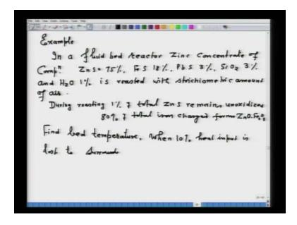
Now, let me give an example to calculate this temperature attainted. So, let me take an example, when I was telling to you about the roasting, I have said at that point of time that there is a fluidized bed roasting. Now, in the fluidized bed roasting, the reaction rate is very fast. Some of the company employs fluidized bed roasting.
