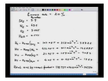
Now here the gases will comprise of SO2, N2 and excess oxygen. The excess oxygen will be equal to 3.065 plus moisture equals to 0.555. The amount is same as it was earlier and there is hardly any change. So, with this modified material balance of the gases, we have to recalculate the H T minus H 298 for nitrogen, oxygen, SO2 and H2O and we can take it from the stoichiometric amount.
