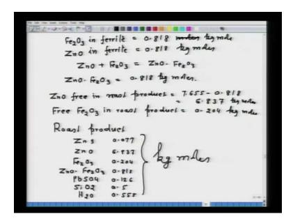
Now, we can find out for Fe2O3 in ferrite and that will be equal to 0.818 moles. ZnO in ferrite is equal to 0.818 kg moles and here also they are kg moles. Now, in these, the reaction, which is to be pursued is ZnO plus Fe2O3 is equal to ZnO into Fe2O3. According to this reaction, material balance has come and therefore, amount of ZnO, Fe2O3 is equal to 0.818 kg moles. ZnO, which is free in roast product will be equal to 7.655 minus 0.818 and that will be equal to 6.837.
