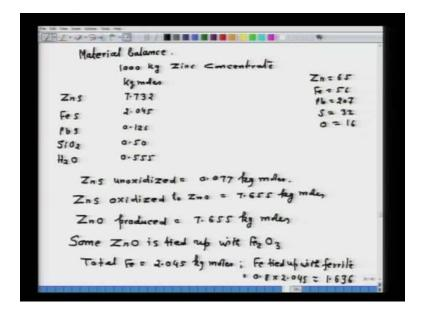
Now, we have to calculate the bed temperature in the fluidized bed. There is a bed, which is in the fluidized state and this is a technology for rapid conversion of sulphide to oxide. As usual, in all heat balance, material balance has to be done first. So, let us take material balance, we have taken 1000 kg zinc concentrate and let me put it kilogram moles. So, I know ZnS, Fes, PbS, SiO2, H2O.
