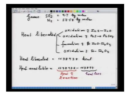
So, with those values, I can calculate heat liberated. Now, heat liberated will be oxidation of ZnS and that is one thing. Oxidation of ZnS to ZnO is the reaction that I have already shown you on this slide. Oxidation of PbS is PbSO4, then formation of ZnO into Fe2O3 is this one and then oxidation of Fe to Fe2O3 has no reaction. So, one can calculate heat liberated because of the chemical reaction. I am not substituting, but you can directly substitute the values.
