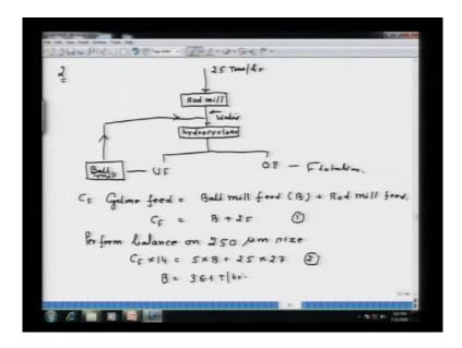
Now, let us see the problem number two: problem number two is as such, say we have a circuit, here is a feed, you have 25 tons per hour, you have here rod mill and from here it goes to hydrocyclone that is was given to you. Hydrocyclone; it separates underflow overflow. Underflow; it enters into ball mill and that further goes to the hydrocyclone for separation and here water can be added. So, the problem says 25tons per hour and this goes to floatation whatever concentration operation.
