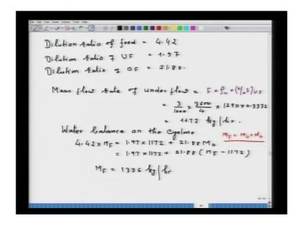
Now, I can find out dilution ratio of feed. Well, I already given the formula, so feed that is equal to 4.42, dilution ratio of underflow that is equal to 1.197 and dilution ratio of overflow is equal to 21.88. Once we determine the dilution ratio, we can find out mass flow rate of underflow. Mass flow rate of underflow will be equal to the formula F into density of underflow into percent solid in underflow.
