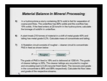
Now, let us take the problem six. Problem six again is a very simple problem; it simply says a plant treats 210 tons of material in a shift of metal grade. This one concentrate in metal grade, tailing metal grade is given, calculate mass of concentrate and tailing.
