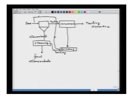
Say for example, if this is the operation, this is the feed, then it goes to scavenger and scavenger tailings are discarded. Now, the concentrate is further subjected to grinding operation as it contains some of the un liberated particle. Now, this grinding is again taken to the feed; from the concentrate, the feed it the concentrate rather enters into cleaning.
