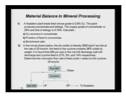
Now, as such, the first problem is a floatation plant treats feed, whose grade is 0.8 percent copper. The plant produces concentrate and tailings, the copper grade of concentrate is 26 percent and that of the tailing is 0.16 percent. Now, calculate copper recovery in concentrate, fraction of feed in the concentrate and c - enrichment ratio.
