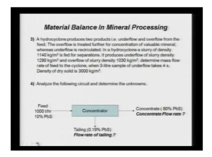
Problem number three: a hydrocyclone produces two products. Now as I have said, the hydrocyclone, it separates feed into overflow and underflow. So again, here two product formulas have to be used. A hydrocyclone produces two products that are underflow and overflow. From the feed the overflow is treated further for concentration of valuable mineral whereas, underflow is re circulated.
