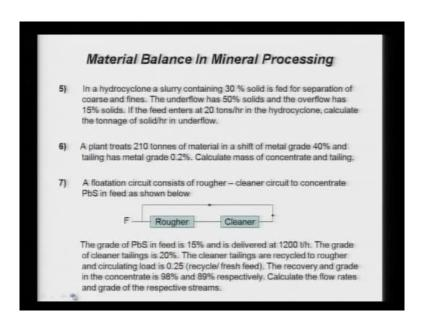
Problem fifth: in a hydrocyclone, a slurry containing 30 percent solid is fed for separation of coarse into fines. You can call coarse as underflow and fines as overflow. Overflow will be taken for further concentration operation; that is, to recover the particle containing minerals. The underflow has 50 percent solids and the overflow has 15 percent solids. If the feed enters 20 tons per hour in the hydrocyclone, calculate the tonnage of solid per hour in underflow.
