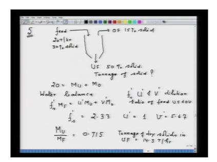
Now, problem number five. This is the say sort of hydrocyclone, we are having the feed which is 20 ton per hour having 30 percent solid. You have overflow, which is 15percent solid and we have underflow, which is 50 percent solid. We have to find out, if the feed enters at 20 tons per hour in the hydro cyclones calculate the tonnage of solid per hour in
