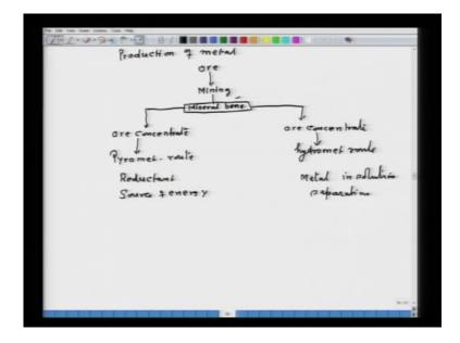
So, let us further follow it up. Let us consider a production of metal from an ore. Let us consider a general flow sheet of production of metal from an ore. For example, I take an ore; whatever the ore from the natural reserve, I have to subject it to mining operation; and this mining operation has to be followed by mineral beneficiation.
