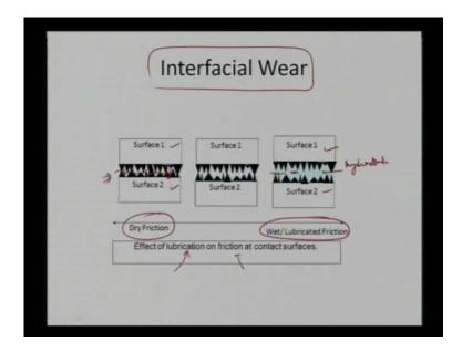
And most importantly, interfacial wear is also one of the very critical components. So, the first we have surface 1 and surface 2. How do they interact, how the how is overall roughness, how is the overall chemistry, how is the overall lubrication lubrication between the two surfaces will result, how my material will now be lost once I have two operating surfaces.
