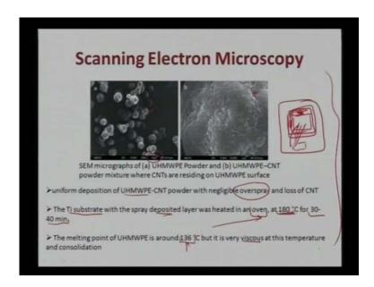
So, from the Scanning Electron Microscopy, we can see that how the powders are being generated. Like, we can see some powder particles which are approximately around 20 microns also. We can see the microns bar here. So, around 10 to 20 micro microns in diameter and then we can also start reinforcing them with some carbon nanotubes.
