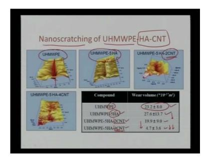
So, we can see how the composition itself can be much more influential in terms of dictating the overall wear between the 2 between the two compositions. In this case, we
