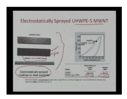
This is how the coatings look like. In this case, we utilize only the polyethylene with some carbon nanotube. So, in this case we have ultra high molecular weight polyethylene and we have around 5 weight percent of multi walled carbon nanotube. And, the coatings show very smooth surface finish as you see here. And, in this case because of CNT, we are seeing a little greyish coating.
