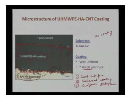
Now coming next, we can see that this is the second case. We have some ultra molecular polyethylene with hydroxyapatite coating. So, in this particular case we have titanium, 6 aluminium, 4 vanadium substrate. And over that, ... spread this particular coating, which is ultra high molecular weight polyethylene. This is now reinforced with some
