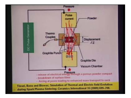
Now, this current will flow either to the graphite dye wall or to the powder compact, depending on the conductivity of the powder compact - porous powder compact.
