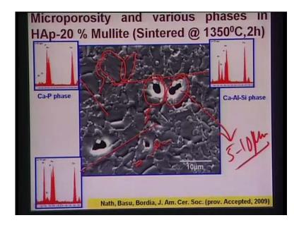
Now, typical SEM image essentially tells to that you have a micro porosity in the structure; and this porosity is roughly 5 to 10 micron in size. And this micro porosity is also associated with certain crane boundary phase, and most likely it is calcium aluminosilicate phase, which is formed along this grain. So, this is your tricalcium phosphate or hydroxyapatite Ca P grains.
