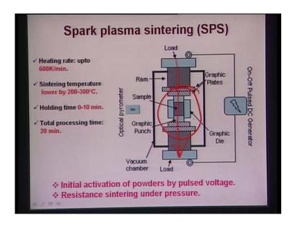
Now, for that we have carried out Spark plasma sintering experiments; and this Spark plasma sintering as I explained to earlier, so it is like a hot phrase by the fundamental
