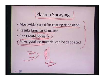
And plasma as we know as the four state of matter here in it is used utilized to basically let the powder through it and it will melt it and it will accelerate the powder particles so, that they get imparted on to a substrate.
