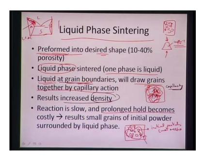
So, solution to that aswe can go with something called liquid phase sintering and in the liquid phase sintering what we are doing here is, first of all we make a particular component and that component is a green and that is preformed into a desired shape. So, we take a particular a particular structure and then we preformed it to whatever kind of a shape in it say if we want to have certain kind of a shape, we basically preformed into certain shape.
