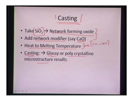
And third process can also be casting, and in this particular case we can take silica which is S i O 2; and S i O 2 is the network forming oxide. So, silicon oxide it basically tends to form network whether itself, so it may not lead to a very all under the crystalline structure it will basically start forming networks.
