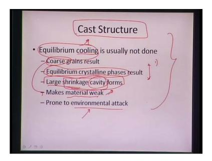
As we had seen earlier that there is we can also provide some casting to get a particular shape and the problem is that the casting is once we are trying to cool the particular material in equilibrium, we get a very coarse material, the grains structure becomes very coarse, though we will get some equilibrium crystalline phases, but the problem will be it
