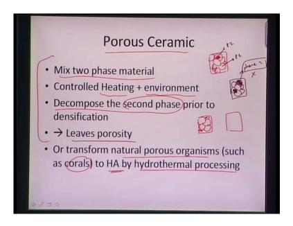
And in porous ceramics how do we get it first of all we will mix two phase material and we provide a controlled heating and with a control environment. So, we have initially two phases: one phase and second phase out here. So, we will have one phase, we have second phase which is basically being embedded into the two phase material.
