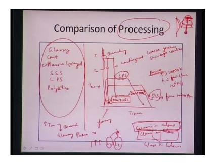
We can see that, we can have a variety of microstructure which which can generate depending on the processing technique. So, we can either of a glass glass glassy kind of a structure, we can also have a kind of a cast structure, we can also have plasma sprayed structure, we can also have a kind of solid state sintered ceramic, we can also have liquids liquids liquid phase sintered ceramic, we can also have a kind of a polycrystalline
