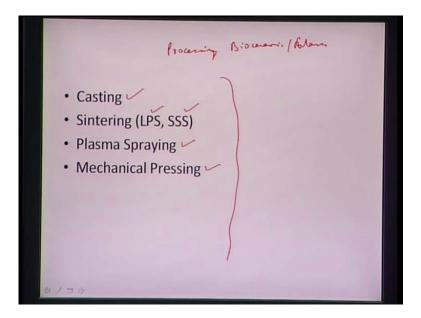
So, that is what we are able to see out here that we can get various kind of techniques for processing the ceramic, bioceramic or a bioglass or a glass kind of a composition either via casting or via sintering which can be liquid phase sintering or can be solid state sintering, it can be again plasma spraying, it so basically thermal treatments are utilized in this particular case and it can again be more mechanical pressing as well to revealed the certain microstructure.
