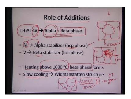
Again, as I said earlier, the role of additions, they go on to titanium 6 aluminum 4 vanadium, it forms a dual phase microstructure. So, alpha comes basically from the titanium part. At the same time, alpha is also being stabilized by aluminum. So, aluminum also acts as the alpha stabilizer. It renders making HCP phase much more stable, but the presence of vanadium helps forming a beta phase. So, we see this titanium 6 aluminum 4 vanadium, it is a combination of alpha plus beta phase.
