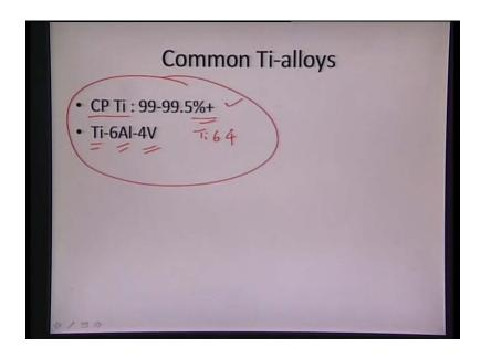
So, that is been widely utilized in the biomedical industry as well as there is a combination of titanium with 6 percent aluminum and 4 percent vanadium. So, it is also called Ti-6Al-4V. So, it is also called Ti-6-4 for easiness in the use, but these are the two some very commonly used titanium alloys which are utilized in the biomedical industry.
