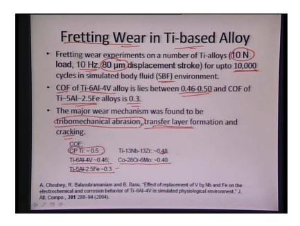
At the same time, they also have done fretting wear of the titanium based alloys. So, fretting wear basically, it was done using 10 newton loads at 10 hertz and for a displacement distance of around 18 microns. They have done, they have gone up to around 10,000 cycles and all these studies were done under the stimulated body fluid environment.
