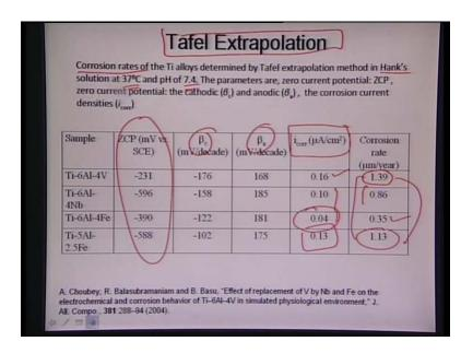
Again from Tafel extrapolation, the corrosion rates were determined for titanium alloys and we can see the corrosion rates in terms of micrometer per year are approximately, similar in nature, whereas titanium 6 aluminum 4 vanadium, showed the best response.
