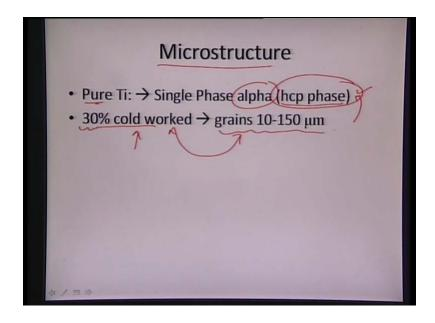
Coming to the microstructure part of it, the pure titanium, it has basically hexagonal HCP phase and the phases called alpha phase. So, pure titanium appears more, it is more of a single phase material and it is HCP and orient to the limited HCP slip place which
