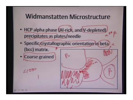
So, we can see this Widmanstatten structure. It is basically, we see that the HCP alpha phase which is aluminum rich and again this is V-depleted in the vanadium part. It starts precipitating as the plate or needle. So, we see that we had grains like this for the beta and then, in that, we see the nucleation of this alpha phase, which can start nucleating at within like this. Then, we have this beta phase and then again, we will see alpha phase
