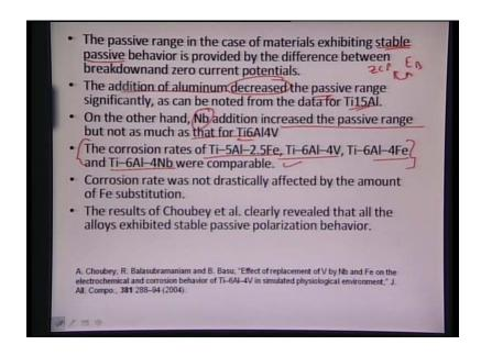
Again, the passive range regime in case of materials, they exhibit stable passive here between the 0 current potential and the breakdown potential and between these regime, they show a much more passive region and we saw that the addition of aluminum basically decreases the passive range.
