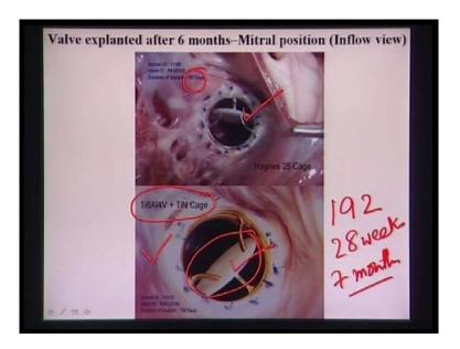
This is the example of this. You know artificial heart valve which is made of this titanium 6, aluminum 4 vanadium that is the alloy plus titanium nitrite coating.
