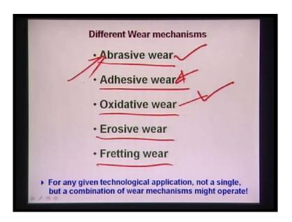
Now, what are the different mechanisms of the wear? Wear can be classified as that 5 primarily distinguishable mechanisms, that is one is that Abrasive wear. Then, it is called Adhesive wear. Then, Oxidative wear and then, Erosive wear. The last one is the Fretting wear. Now, for any given technological applications, it is important that not a single, but a combination of wear mechanisms might operate.
