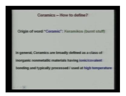
Now, the origin of the word ceramic is derived from the Greek word keramikos. That is, burnt stuff and this ceramics are broadly defined as a class of inorganic nonmetallic materials having ionic and coherent bounds and typically processed or used at high temperature. This is like very formal definition of ceramic base materials.
