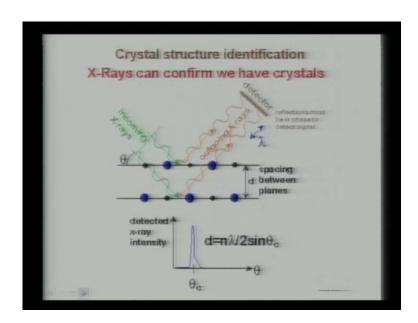
Now, how the structure can asses in a particular material. One of the simplistic way to use that extra diffraction. So, this extra diffraction means, like, if there are two parallel atomic planes, then if the incoming x rays are coming here, now they will be diffracted by the atomic planes. This diffraction based on this; what is angle of diffraction, then you can find out, there is bragg's law which is, n lambda is equal to 2 d sin theta.
