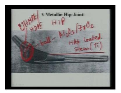
Now, this is a thing that I was mentioning new couple of minutes ago. Now, this is called stem. Now, this stem is typically made of titanium. On this titanium, you can put the hap coating also. Like you know, hap coated steel titanium also you can use. Now, this is the part, longer part of the structural part or load varying part of the stem total hip joint; so,
