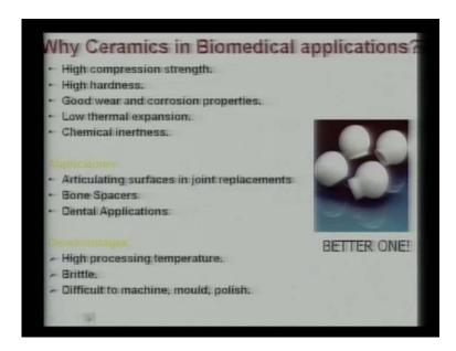
What are the important properties which are of relevance for ceramics and biomedical applications? That includes high compression strength and high hardness of these materials. It also is a good wear and corrosion properties. Applications, it can be used articulating surfaces in joint replacements, bone spacers, as well as the dental applications.
