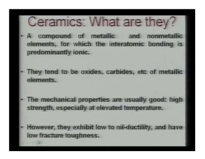
Now question is that, what are Ceramics? Ceramics, is essentially a compound of metallic and nonmetallic materials nonmetallic elements and for interatomic bonding is primal predominantly ionic.
