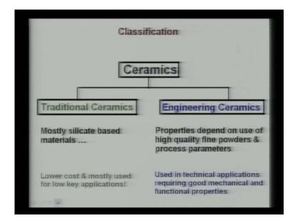
So, that means, that it has a pure inorganic material and it has ionic or coherent bonding. They are typically used or processed at high temperature. Now, ceramics can be broadly classified into traditional ceramics and engineering ceramics. But, as per biomedical applications are concerned, we will be mostly dealing with engineering ceramics like alumina and zirconia, where that properties are also depend on high quality fine powders and process parameters.
