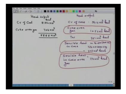
So, if we do that we will consider say energy input or we can call heat input whichever, way you want to understand. So, heat input was calorific value of coal and that is equal to 8184 into 10 to the power 3, these values are in kilo calories. Now, also coke oven gas because 40 percent of coke oven gas is burned, so accordingly the heat which is entering is 704 into 10 to the power 3 kilo calorie, and that makes a total 8888 into 10 to the power 3 kilo calorie as the heat input.
