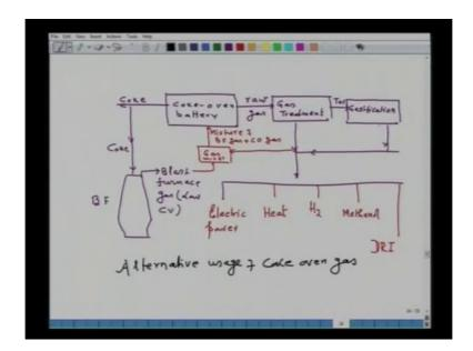
Now, in order to show this possibilities, let me draw a sketch for you, so that you can understand now for example, we have the coke oven battery, say this is the coke oven battery (No audio from 45:07 to 45:16), the coke is being produced, now coke and of course, it is used in the blast furnace (No audio from 45:30 to 45:43), so here this is the blast furnace and here the use of coke, now we have air blast furnace gas low calorific value. Blast furnace gas has a very, very low calorific value.
