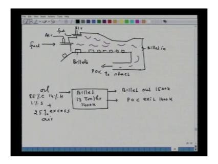
Now, for example, the furnace looks something like this is a belt on which there is a continuous discharge of the billet enters and exits. This is the burner, this is another burner it is somewhere here, there is a billet in, here P O C to stack, here you have billet, they are moving continuously and here billet is out, here supply is fuel and here supply air same thing here fuel and top is supply air.
