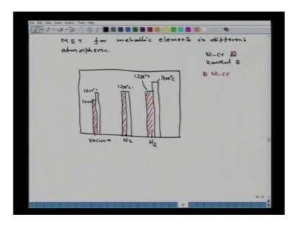
So, let us consider now say maximum element temperature for metallic elements for metallic elements in different atmospheres in different atmospheres, again I plot here, I have taken two thermo couples two heating elements, one is the nickel chromium, that is nichrome and another is the Kental. So, under vacuum, say (No audio from: 30:49 to 30:58) under vacuum this one say this one is in fact, nickel chromium whereas, this one is the Kental.
