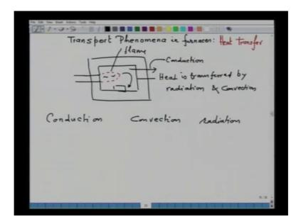
So, for example, if we consider a combustion chamber of a furnace which is lined with the refractive material and here we have a burner and this burner produces a flame. And here we have the charge so, this is the flame and the product of combustion transfers it is heat to the charge to the combustion chamber and hence heated up. Part of the heat is also transferred to the surrounding and hence heat losses are important. Therefore, for an efficient furnace
