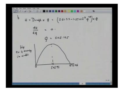
So, in the b part, you have to find out H power equivalent. So, all that you have to multiply drafts into q is the flow rate, that is equal to 261.33 minus 1.27 into 10 to the power minus 3 q raise to the power 1.8 into q. So, we have to find out the god this equation shows there is a maximum.
