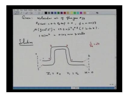
So, this is a typical problem for design of the flue and stack and so on. Now, there is something which is also given. What is given is as follows say, given molecular weight of flue gas is 29, then e f contraction 0.4, e f expansion 1.0, f is given 0.0037 this viscosity in gram, but centimeter per second can be calculated. Sum this relation 19.3 into 10 to the power minus 7 t raise to the power 0.8, where t is in kelvin and 1 Newton per meter square, that is equal to 0.02 millimeter of water.
