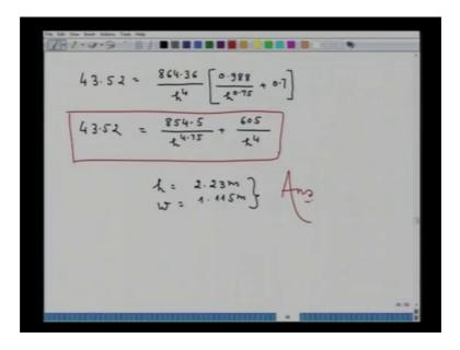
So, I will be getting 43.52 and that will be equal to 864.36 upon h to the power 4 and simplifying, then I am writing I requested to do the remaining exercise at 0.988 upon h to the power 0.75 plus 0.7. So, I get an equation which is to be solved that is equal to 854.5 upon h to the power 4.75 plus 605 upon h to the power 4 and that is equal to 43.52.
