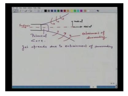
So, if I can represent say this is my burner is a central line. So, here and passing a mixture of fuel plus air and as this fuel and mixture is discharged through the burner, then a free jet is produced. In the free jet, this is called potential core.
