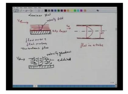
So, depending on the flow, the various type of flow pattern can be seen. For example, we consider the flow a laminar flow of (()) on a flat plate, if I consider this is a flat plate this is the flat plate and imagine the flow is occurring perpendicular to the plate. So, this is the direction of flow of velocity V infinity. So, as the flow comes in contact with the surface immediately one has so called a retarding influence that is the induction of the so called boundary layer.
