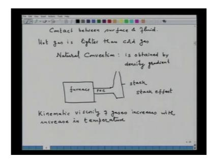
Another important thing is also the contact the contact between surface and fluid. Heating will occur only wherever the fluid makes contact with the surface, no contact no heating will be there. Also important to know that, near this surface, the heat flow will occur will always occur by conduction. And also to know that a uniform velocity of the gas will give you a uniform heating. Therefore, the velocity of gas moving velocity of gas is an important issue.
