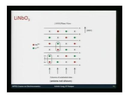
I am just going to show you the cross section of 1 0 bar 1 0 plane. So here, you have again A B A B A B layers. These are the oxygen layers. In between them, you have, so lithium niobium cross, which is the vacant site, then again lithium niobium vacant site. Then in the next layer, since the vacant position moves in this direction, in all the structures, so you will have again niobium vacant, lithium niobium and then again you will have vacant.
