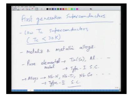
And these first generation super conductors were essentially metals or metallic alloys and they are typically called as essentially low temperature or low T c super conductors; and what do you mean by low T c super conductors is essentially the T c is lower than 30
