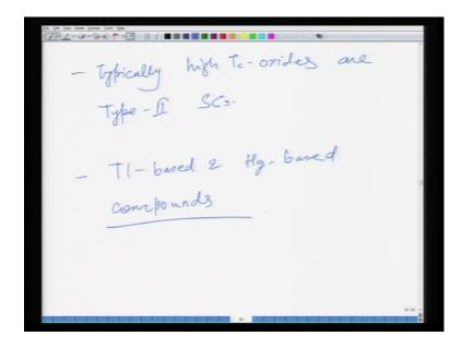
So, you can say that typically high T c oxides essentially most of these are oxides are type two super conductors, but the theory of the physics of operation or just like you have a B C S theory put forward to explain low temperature super conductivity. The super conductivity in these materials is not very well understood; there have been some theories which have been proposed; essentially again quantum mechanical theories, but they have not been successful in explaining it completely.
