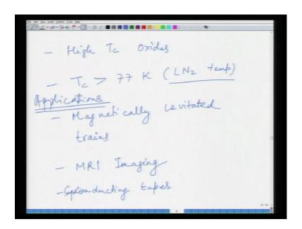
Now, these super conducting oxides since the T c's are typically higher than 77 Kelvin which is liquid nitrogen temperature they have been thought of their used in variety of applications; and these applications could be you know like magnetically levitated trains; you can have MRI imaging; you can have super conducting tapes.
