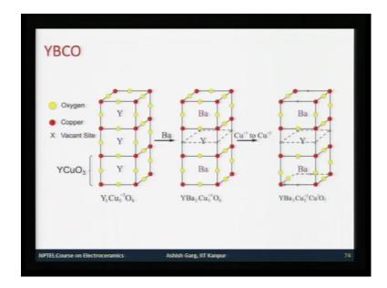
So, the structure changes like this. So, you have this Y 3 Cu 3 O 9 followed by Y Ba 2 Cu 3 O 8 and then Cu 3 plus to 2 plus formation of Y Ba 2 Cu 2 2 plus Cu 3 O 7. So, structure remains similar orthorhombic structure, but what you have here is as a result of these substitutions and reduction in the oxidation state. What you have here is vacancies of oxygen and these crosses are nothing, but vacancies of oxygen, and this also leads to change in the coordination of copper atoms.
