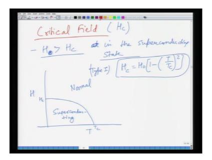
So, another concept which comes in the wake of this Meissner effect is called as critical field and this critical field is essentially H c. So, when H is greater than H c then you can say in the super conducting state the material does not remain super conducting.
