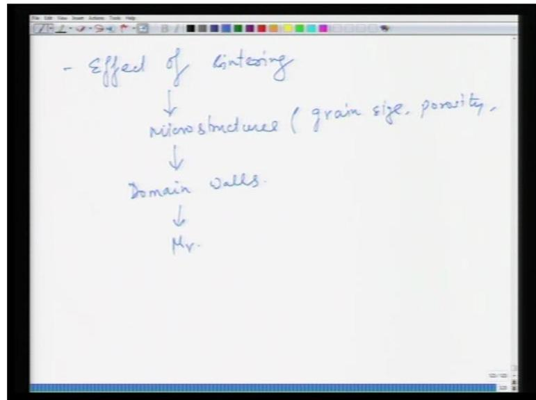
So, so you can have effect of centering. Now centering as you know is a densification process and this densification process the way you carry out what temperature, what atmosphere, what time. This determines the densification of the ceramic and this densification essentially controls the micro structure. Micro structure will mean grain size porosity grain size would mean grain boundary as well and the type of grain boundaries whether they are insulating, whether they are conducting etc
