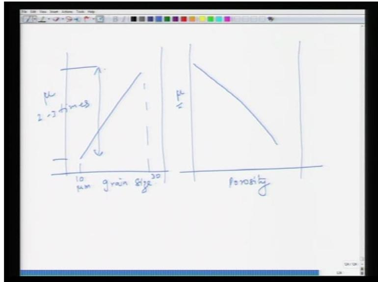
So, for instance, so if you look at for example, in some system the variation of  $\mu$  as a function of grain; size the model system then it increases as you increase the grain grain size from. Let us say 10 micron to something like thirty microns and this increase in permeability can be two to three times. So, this is the effect of grain size and then you can also do it by. You can also study the effect of change of fractional porosity. So, porosity also has a dominant effect.
