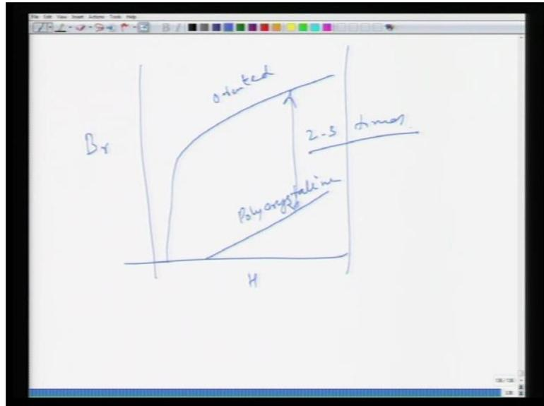
So, for instance if you look if you plot the magnetic induction  $B_r$  versus  $H$ . So, for a for a polycrystalline the behavior would be something like this and for oriented barium hex ferrite would be like this. And this would be at least three or two times change in the in the in the properties.
