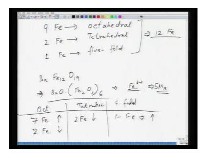
So, coming back to magnetic characteristic now, you have 9 iron atoms going to octahedral sites, out of 12 and 2 iron atoms going to tetrahedral sites and 1 atom remain 5 fold coordination. So, this makes up 12 Fe and the formula is B a Fe 12 O 9. So, essentially it is going to be, Ba O dot Fe 2 O 3, into 6. So, this is how the structure is essentially and now you can also see why it is like, why it is like a mixing of hexagonal
