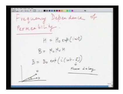
So, we said that just just like you have in case of electric field, you have simultaneously sinusoidally varying a c electric field, you have a magnetic field, which is also similar in the form H is equal to H naught exponential of i omega t and this since, now you know
