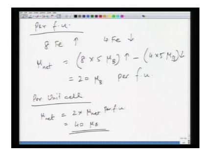
So, basically per formula unit 8 Fe spin up and 4 Fe spin down. So, mu net would be 8 into 5 mu B spin up minus 8 into sorry 4 into 5 mu B is spin down and what this gives rise to is essentially 20 mu B per formula unit. So, essentially what you have is, 20 Bohr magneton of magnetic moment per formula unit of barium ferrite. Now, for per unit cell
