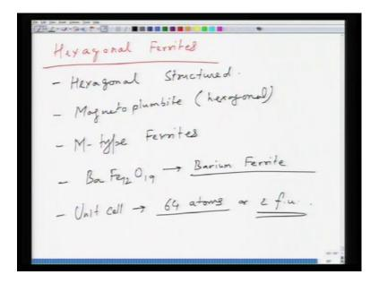
Another category of magnetic ferrites is hexagonal ferrites. So, as a name itself suggests these are hexagonal structured and parent structure for these compounds is basically magneto plumbite, which is hexagonal compound and typically you call these materials, they are also called in literature as M type ferrites. M type comes from magneto
