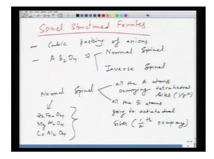
So, essentially what you have is A B A B 2 O 4 structure. So, you can have normal, you can have inverse spinel. In case of normal spinel, you have, which means one-eighth occupancy and all the B atoms going to occupancy. The example of normal spinel structures could be your zinc ferrite, magnesium aluminate, cobalt aluminate etcetera and inverse spinel.
