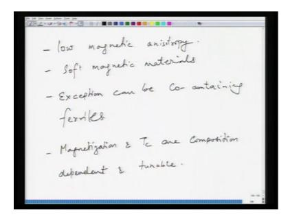
Another thing that you find in spinel, perovskite spinel, cubic spinel, ferrites is that that they have low magnetic anisotropy, which means they do not have a strong dependence of magnetisation on the crystallography. So, as on the crystallographic directions, so as a
