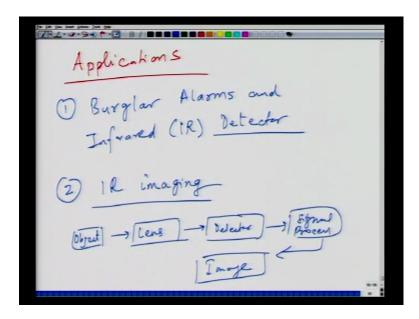
Another application could be IR imaging. Not only the pyroelectric materials can be used as alarm or detectors, they can also be used for imaging a particular, let us say, a body. The principle here is because the body has different parts and all of these parts are at
