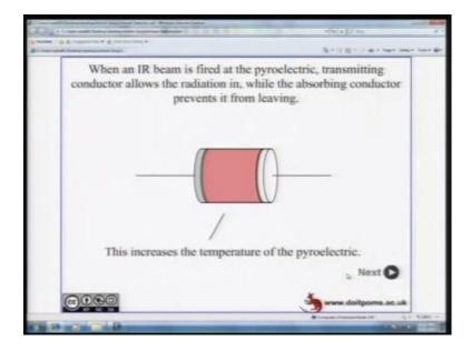
And, when you put them together, they look like... And, when you send an IR pulse to this material; naturally, this IR pulse is nothing but it is a long wavelength radiation, which represents the ambient. And, this increases the temperature of the pyroelectric.
