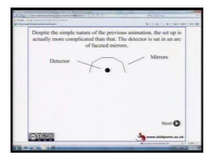
The set up of this; although it looks pretty simple on the paper, but the set up is quite complicated. So, basically, how you make the detector is it is put in an arc of faceted mirrors. So, you have these faceted mirrors, whose job is to reflect the radiations, so that the reflected radiations are not lost.
