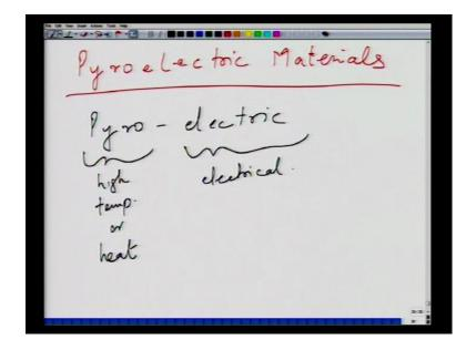
Now, the third class of important material in this non-linear dielectric category is pyroelectric material. Now, as a name itself suggests, you have pyro and then electric. Pyro essentially means high temperature or temperature let us say heat — or heat. And, electric means electric — something do with the electrical things. So, it is the coupling between thermal and electrical things, which gives rise to what is called as a pyroelectric effect.
