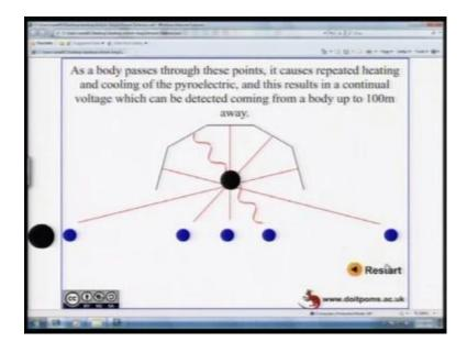
As a result, you have large signal, which results in large heating or repeated heating and cooling of pyroelectric. As a result, you have a continuous voltage. And, this has a sensitivity of up to 10, 100 millimetres, 100 meters. So, this is one application, whose animation just now you saw.
