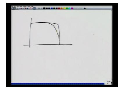
And, depending upon also the nature of transition, for a ferroelectric material, you can have a sudden transition in the polarization or you can have a gradual transition in the polarization. So, depending upon whether you have first order or second order transition, the magnitude of delta P i will also be different for both of these different kinds of effects.
