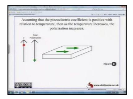
As a result, assuming that the piezoelectric coefficient is positive with respect to temperature; which means, then, as the temperature increases the polarization increases. So, as you increase the temperature, you are increasing the strain; which means polarization is increasing. So, this is what you see here. This is as you increase the temperature, the overall polarization has gone down; but, this piezoelectric term has increased the polarization by some magnitude.
