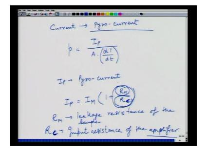
Basically, this current is essentially, which passes through an amplifier, is called as a pyro-current. And, pyroelectric coefficient as a result, is given as I P, which is a pyro-current divided by A – area divided by dT by dt. So, rate of change of temperature. So, I
