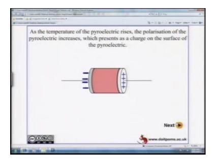
As a result, you develop a polarization on the surface of the pyroelectric.
