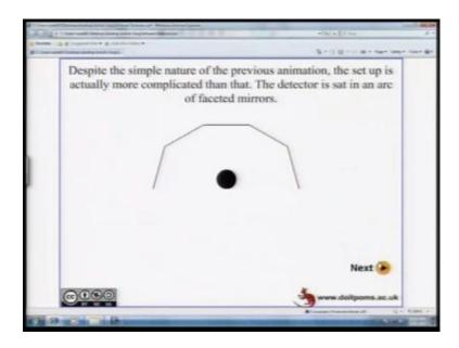
These are the... So, this is how it looks like. You have this detector, which is sitting inside this arc or a shape, which is made by the faceted flat mirrors.
