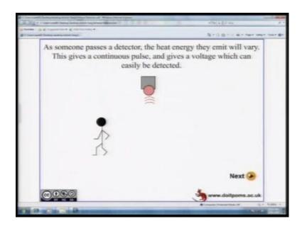
As someone passes in the vicinity of this detector, the thermal energy, which the humans or the object will emit – this will vary and this will give rise to a pulse. So, it is like a pulse IR radiation. And then, this generates a voltage, which can then be easily detected.
