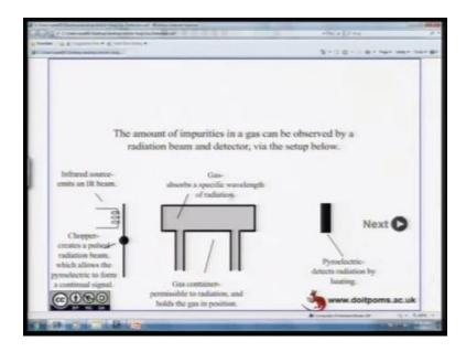
The amount of impurities in a gas can be observed by a radiation beam detector using the setup, which is shown below. This setup has an IR source, which emits an IR beam. And, you have the gas, which absorption characteristics towards specific wavelength of radiation and which is inside a container. Then, a pyroelectric, which detects radiation by heating.
