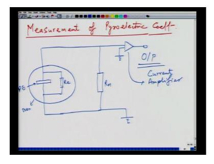
Now, how do you measure the pyroelectric coefficient? Because the moment you know that, it is an important quantity, you need to revise methods how to measure it. And, one
