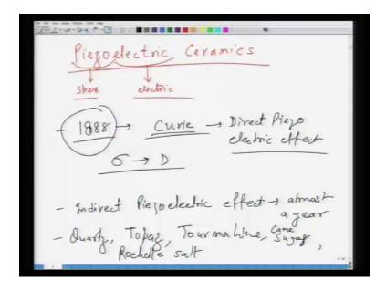
Now, the topic of this lecture is essentially piezoelectric ceramics. Now, piezoelectricity is basically an interesting effect, which is essentially, if you look at two terms: piezo and then electric; piezo relates to stress or force – piezo; and then, electric means you have electric. So, it is coupling of stress and electric field or coupling of mechanical parameters with respect to electrical parameters. And, this is what makes these materials
