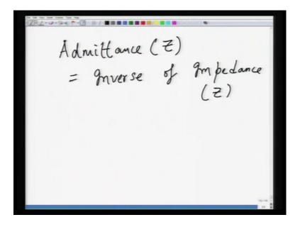
So, admittance, let us define as admittance Z, this is inverse of, let us say impedance. Impedance is nothing but as you can, as you can understand from these term itself. Impedance impedance means the overall resistance of the material, admittance is nothing but something which is related to you know admitting. So, admittance is nothing but really opposite to inverse of impedance.
