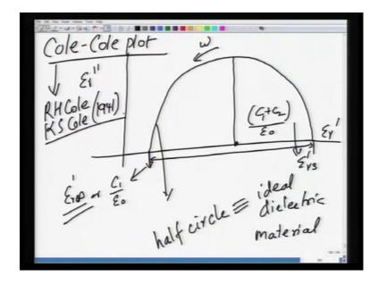
If you just, if I just write it slightly away, so that it does not get confusing epsilon r prime. So, this value becomes epsilon prime r s, which is the because in we are increasing the frequency in this direction, a static dielectric constant and this becomes your... So, or alternatively, in terms of electrical circuit, this becomes equal to C 1 plus C 2 divided by epsilon naught and this becomes or C naught depending upon, how you say?
