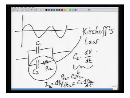
Then as a result of the nature of this this wave form your capacitor will charge and discharge and charge and discharge. Now, so based on that, if you, so if you apply this to the R 2 C 2 element, so you have C 2 C 1 C 2 R 2, so here what happens is, this capacitor C 2 charges through this resistor R 2. Now, what we need to do is that, suppose suppose we apply a field to this particular segment, we can apply, what we call as Kirchhoff's law to this segment. So, we apply Kirchhoff's law.
