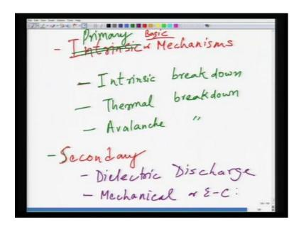
So, these these failures are often you you you divide them in two categories. One is the intrinsic mechanisms and these intrinsic mechanisms are nothing but your defined as, or or rather intrinsic or basic mechanisms. So, one is called as intrinsic break down, then you have thermal break down. Instead of intrinsic, let us call it primary, primary mechanisms, because these two intrinsic clash with each other. Then you have avalanche break down, and then and you have, what is called as secondary.
