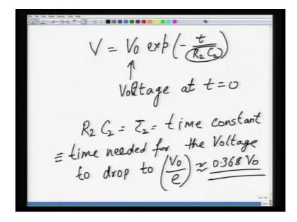
So, if V naught is the voltage at t is equal to 0, R 2 C 2, which is in the exponential term must have same units as of time. This R 2 C 2 is defined as tau 2, which is called as time constant. This time constant is basically the time, which is needed. So, this is nothing but equivalent to time needed for the voltage to drop to a value V naught by e, which is, which comes out to approximately 36.8 percent of V naught, so or 0.368 of V naught. So, tau 2 basically is the time.
