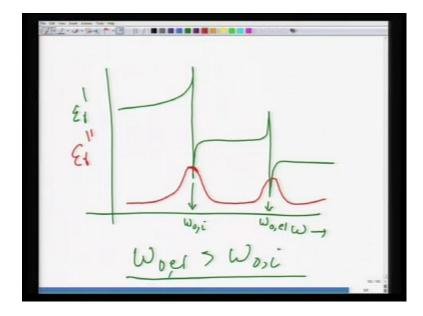
And if you if you plot epsilon r double prime, this shows loss at these frequencies. So, this undergoes a maxima in the loss, characteristic maxima. So, this is this is when they absorb maximum energy, as a result the loss is maximum. So, this is typical of these two mechanisms, where you can consider a charge dipole as a linear oscillator.
