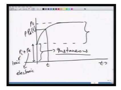
And this happens to be in the range of Mega Hertz or so. And as a result the way polarization develops is. So, when you plot the polarization as function of time, you have an instantaneous development of polarization component which is nothing but sum of ionic electronic. Because you know that electronic ionic mechanisms are extremely fast.
