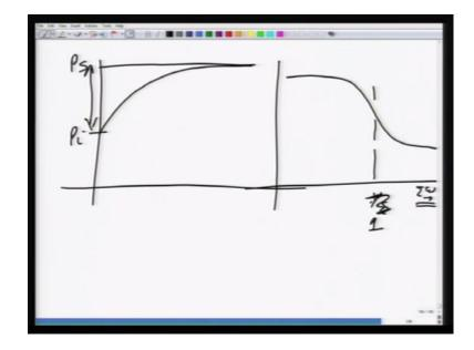
Which goes as, so it develops into P s a little bit slowly from P i to P s, it takes bit of time. And as a result of this, you have when you plot dielectric constant. It goes like this through a frequency 1 over tau, and or if you plot omega versus tau, if you plot frequency is 1 over tau, but if you plot omega tau then it becomes equal to 1.
