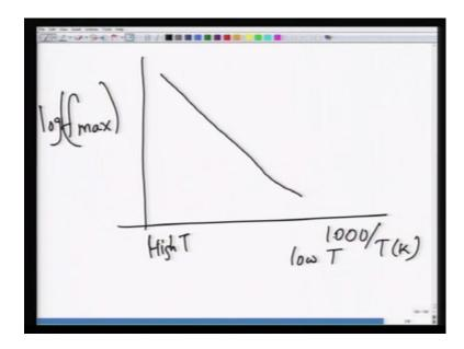
You can also plot this f max log of f max versus, and as you can see that this would be as the temperature is as the temperature is. So, this is your low temperature, high temperature side, this is your low temperature side. So, at higher at higher temperature you will have f max occurring at higher frequencies whereas, at lower temperature Maxwell occur at a lower frequencies, because the relaxation time will be larger at these frequencies. So, the complete picture is now rather different.
