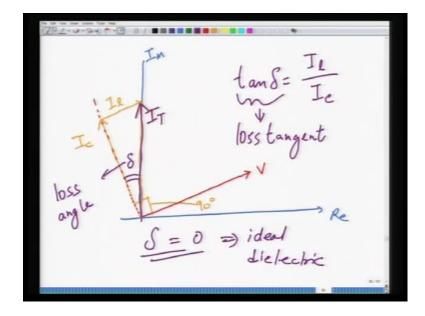
And what we do the next is and now basically this presence of this loss current how how how can it be schematically shown? So, if you have so this if this is the voltage in the charging current, which is 100 percent current the ideal ideal dielectric leads the voltage by 90 degrees. In addition you have a loss current which is in phase with the applied field and which is depicted by this vector. Sum of these two vectorial sum of these two I c plus I1 gives rise to IT.
