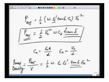
Higher it is higher would be the average dissipation of, average power dissipated and you can see that this is equivalent to writing half V naught square omega C d. C d is a capacitor of a dielectric multiplied by tan delta. So, higher omega is higher P averages and higher tan delta is higher the losses. So, basically it scales with tan delta so higher the loss factor is higher the power dissipation would be.
