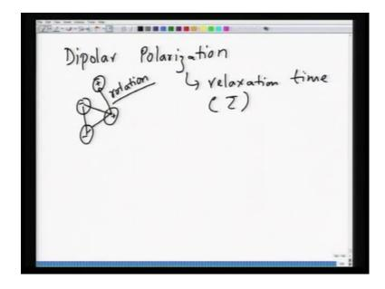
Then third polarization mechanism that we looked at was dipolar polarization. Now, in case of dipolar polarization you have a molecule like this. So, let us say this is minus, this is plus and this goes from one state to another state where this rotates, let us say.
