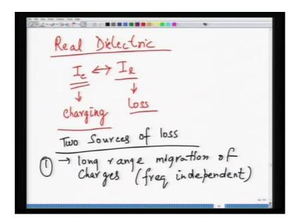
So, as a result they have certain loss in terms of charges storage. So, what basically means is that some sort of the charge leaks out of dielectric material and which is represented by a quantity called as dissipation factor or loss factor.
