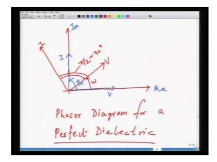
So, this is the phasor diagram for a ideal dielectric where current leads a voltage by 90 degrees and this results in 0 power loss.
