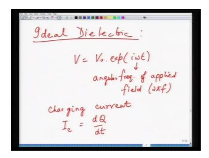
And we looked at the case of ideal dielectric, where power dissipation is 0 and current leads the voltage by 90 degrees.
