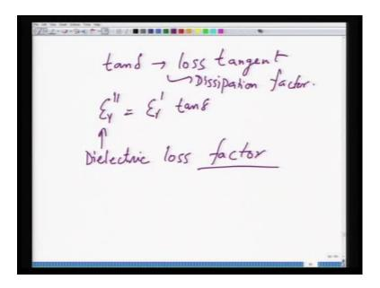
So, tan delta is often called as loss tangent or dissipation factor or epsilon r double prime is called as dielectric loss factor which is which is product of epsilon r prime and tan delta. So, naturally higher tan delta is higher epsilon r double prime would be.
