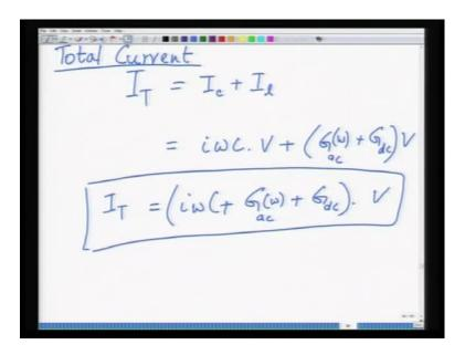
So, the total current in for a real dielectric would be charging current plus loss current and as a result we get an expression for this.
