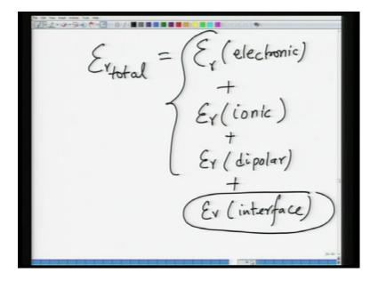
Now, so the first polarization which... So, the dielectric constant of a material is, so in general dielectric constant total epsilon r total, this can be written as sum of epsilon r electronic plus epsilon r ionic plus epsilon r dipolar plus epsilon r interface. Now, usually interfacial polarization is an extrinsic effect, that is why when we make calculations of dielectric constant. We take the first three things into account not the last thing last thing.
