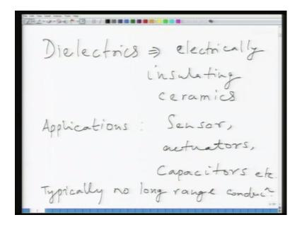
And, so what we will do is that, first we will look at; or maybe I will first, so dielectrics are electrically insulating ceramics, and they are used in variety of applications as I said; sensors, actuators, capacitors, etcetera, plenty of applications depending upon the type of the ceramic and typically no long range conduction.
