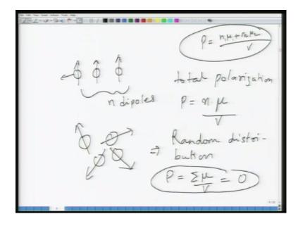
And if the dipole strength was different, then it would be P is equal to n 1 mu 1 plus n 2 mu 2 etcetera, divided by whole volume. So, this would be the case if the dipoles
