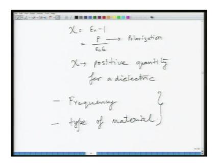
So, chi is equal to epsilon r minus 1, and what this would be equal to P divided by epsilon naught E. So, what basically dielectric susceptibility is, basically dielectric susceptibility is nothing but ratio of polarized charge. So, this P is nothing but polarization or polarized charge, divided by the charge surface, charge in a vacuum capacitor. So, polarized charge or the excess charge divided by the charge on the surface of the vacuum capacitor.
