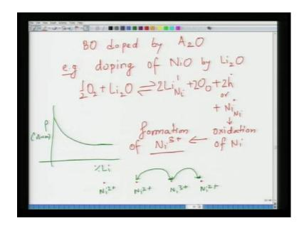
Then we looked at the case case for example, how does the resistivity changes in ionic solid for example, in a doped oxide.
