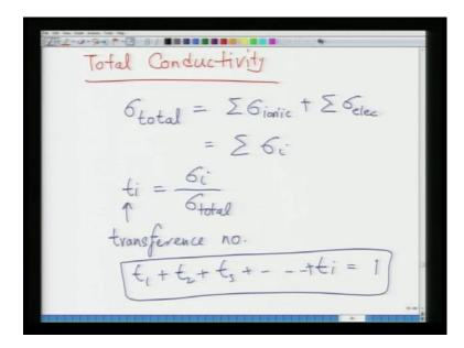
We looked at a transference number and this transference number is nothing but ratio of ionic or electronic conductivity to the total conductivity, so any type of conductivity divided by total conductivity because total conductivity is sum of all source of conductivities. So, for a perfect ionic conductor t will be equal to 1, t ionic will be equal to 1 and for perfect electronic conduction t electronic will be close to 1.
