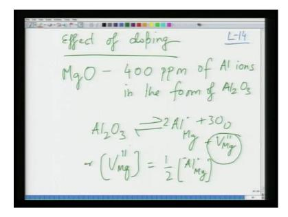
So, and effect of now this is because magnesium oxide is prone to having impurities so it contains about 400 PPM of roughly aluminium ions, in the form of A 1 2 O 3. So, now you can write the defect reaction as you can. So, A 1 2 O 3 going to so A 1 going to M g site and it is going to give rise to one positive charge. So, since both the aluminium's go
