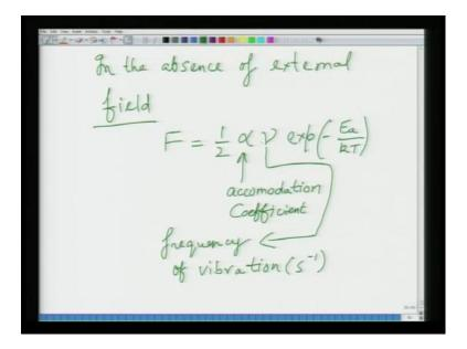
According to Boltzmann statistics, the probability is equal because the barrier is equal. So, let us say the probability is F. So, F can be given as half. Half is the factor because it can move to either side alpha. Alpha is let us say some some coefficient called accommodation coefficient multiplied by nu. Nu is the natural frequency of vibration or where vibrational frequency, multiplied by exponential minus of E a by k T. So, this is your typical Boltzmann equation.
