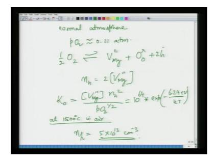
So, at 1600 degree degree centigrade in air, I can calculate using this expression. From this I I can calculate what n h would be and this n h works out to be 5 into 10 to power 13 per centimetre cube. This whole concentration works out to be much larger than the a electron or whole concentration, which are thermally generated, which are of the order of 10 to power 9. So, we will ignore those.
