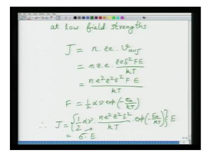
Low field strengths we can write current density as J is equal to n into Z e into v average which is nothing but drift velocity. So, now this would be n Z e multiplied by delta square what we wrote in the previous slide was Z e delta square F E divided by k T. So, this becomes equal to your n e square Z square delta square F E divided by k T. So, now
