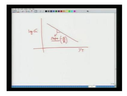
So, you can see that resistivity or conductivity has similar relation to temperature as diffusivity has. Simply because proportional to and again proportional to diffusivity and similarly, just like diffusivity it also has extrinsic intrinsic regions.
