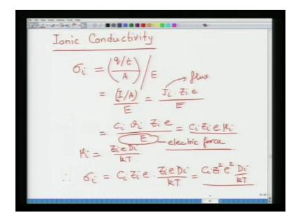
Then, we looked at what is ionic conductivity in these materials. Ionic conductivity is nothing but C i, Z i, e, mu i and you know what mu i is mu i is nothing but the ionic mobility.
