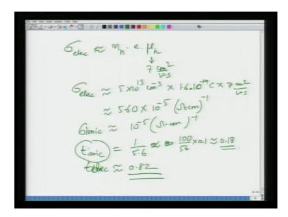
Now, if you calculate the electronic conductivity, sigma electronic this will because the electron concentration is very small as compare because thermally created electron hole
