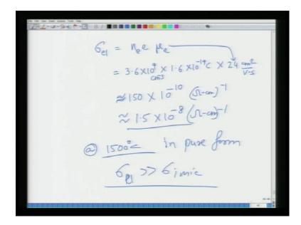
So, what we found in this example was that in the pure form at 1500 degree centigrade, sigma electronic is much larger than sigma ionic. So, what we will do in these classes is, we will look at what is the effect of doping on conductivity.
