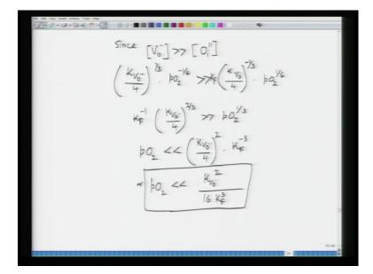
And then you can determine what is the concentration of all the defects and then I can work out since V O is much greater than O i, I can work out what is the p O 2 condition at which this should happen. So, this is first limiting condition.
