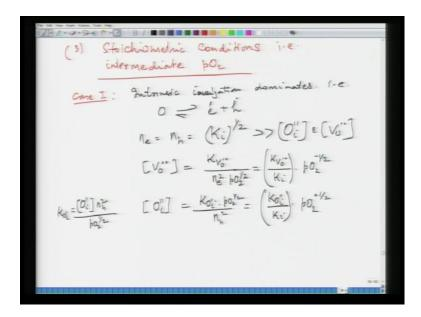
In that case we take two conditions, case one when intrinsic ionization dominates, that is intrinsic creation of electrons and holes. In such a situation, the electron and hole concentrations are equal they are equal to k i to the power half and these two concentration are much larger than oxygen interstitial and oxygen vacancy concentration.
