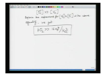
And then we work out what is the what is the regime of partial pressure of oxygen, which is given in terms of k k's of different reactions. So, p O 2 must be larger than 16 k F cube much larger than 16 k F cube divided by k O i square and then the last region which is remaining is the stoichiometric condition.
