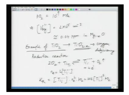
Now, if you change the partial pressure of oxygen. So, if you take p O 2 is equal to minus sorry if you take p O 2 to be equal to 10 to the power minus 9 minus 9 M P a in such a situation again, you recalculate and this gives to V M g concentration of about 2 into 10 to the power 15 centimeter, per centimeter cube. This is equivalent to 0.04 PPM in M g 1 minus x O. So, if you compare these two values, in previous case we got 0.0,
