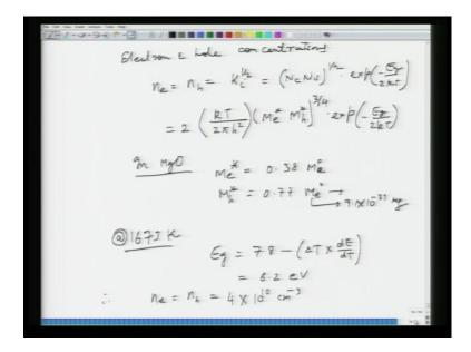
So, we know that n e is equal to n h is equal to k i to the power half which is equal to N c N v to the power half into exponential minus E g by 2 k T right and this would be given as 2 into k T to the power 2 pi h square into M e star into M h star to the power 3 by 4. So, exponential minus E g by 2 k T. So, what I have done is if you go to previous slides n N c and N v were equal to yeah.
