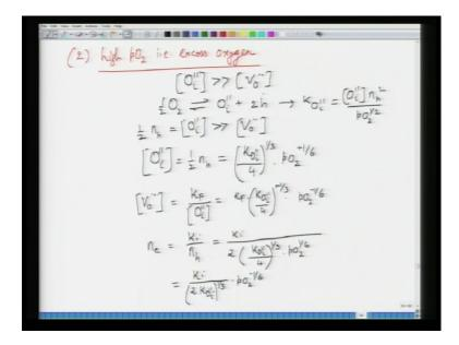
Second limiting condition would be in high pressure region. So, in this case opposite prevails that is oxygen interstitials are much larger in concentration than oxygen vacancies, again write down the charge neutrality condition and write down derive the concentration of all defects.
