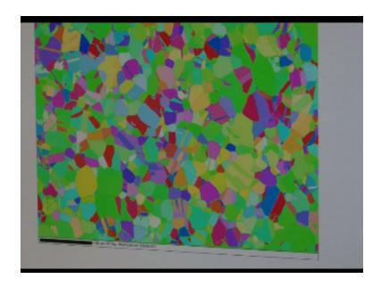
We go down and once you take the information from different grains which are present in the sample after collecting the HD patterns and we can this process in the software and then we can plot it in terms of the gain orientations and this is the quake in the orientations are sown by different colors this each color indicate.
