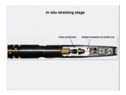
Rather kind of stage another kind of where other holder used in the real microscope experiments you know experiment is called straining stage this one is taken from high citron tanks to them. So there is a holder where actually one can actually do nano indecent test inside the transmission electron column what you see is a basically the sample mounting stage and this is the in and tar and this is position.
