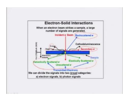
As I shoed this is picture slide I have showed in the beginning of this discussion on the microscopic techniques as a electron forms on a sample in generates all kind of signals you can have a secondary electrons or you can have a backscatter electrons which are based under you can have as x rays or you can have Ager electrons or you can have a Cathodaluminescence on the coming from the tops of the sample one of the electron is falling.
