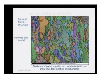
This is just one such picture what I am showing you this is as you see the different grains are mapped with different colors okay this is how the data is this is taken from one of the hk software manufacturing company in UK the oxford instruments we have the facility installed in our microscope is again oxford instruments.
