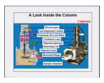
Compare 200 or 300 k volts we are going to continuous from 20 to 40 k volts and not only that the imaging basically imaging is totally different as compare to transmission electron microscope here. So what you see basically is electron guns source which can be either a tan stein or lab six or FEG the fill a machine gun which is normally used nowadays and then this is basically aligned a focus are there be using a lens assembly the condenser lenses.
