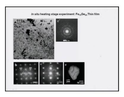
And as you see it alone and this temperature 773k that is approximately 5000C temperature, so you see this whole thin film has been crystallize and this ring diffraction patters source the dual nature, so therefore if you want to do such kind of experiments in the inside a TM column we need to have a to take the diffraction patters at the along with the bright filed or dark field images, so once this thin film is fully crystallize at 773k it can cool down by switching of the Furness.
