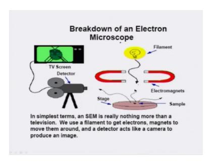
That is what I can say you so there is a filament which gives electrons and there is a sample electron falls interaction a sample and obviously the electron beam can be focused by using electro magnets which just nothing but the objective lens and then after this interaction of the electrons which arte the sample we generate signal the signals can be process using different kind of detectors.
