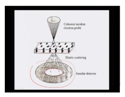
Suppose this is the specimen here as you can see and this is my converge beam coming from this objective lens, STEM and then obviously electrons are undergoing diffractions. See if you use a detector which is angular type, so what actually happens is that we can collect the diffraction information in a disc okay surrounding by this central circle and this is what is called as the angular detector in fact the reasons for it, which I will tell you in few minutes time.
