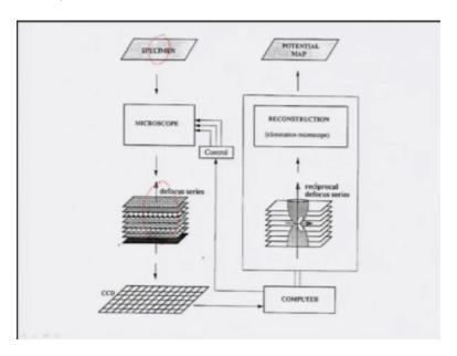
You see their electrons from the gun falls on the specimen after going to do different you know lenses and then interacts interaction basically dynamical in nature and then is basically passes through the other lenses in the microscope like intermediate lenses and finally obtain a image in a CCT camera and to make like this simpler we always get a defocus series of images where
