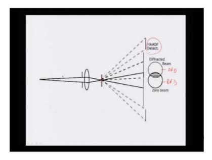
In to the microscope or into the stem is known as HAADF high angular detector, this was basically done or developed by and they have seen that if we use angular detector, angular detector means, it is like this.
