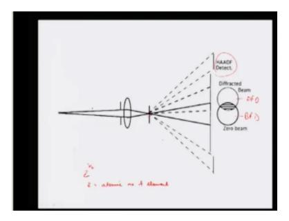
So this is another advantage of the stem, the stem actually as changed the whole color of the electron microscope so much now as I said that the one of the advantage of this higher detectors to obtain z contact images but it has its own you know limitations also limitation in the sense that it has to be properly sample as to properly oriented and many is not fond that very signal are depended on sample thickness the sample thickness is high.
