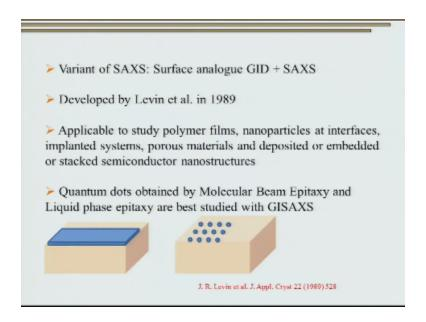
So as I had already mentioned grazing incidence small angle x-ray scattering is a variant of small-angle x-ray scattering but it is used extensively for carrying out characterization on the surface it has it was developed by Levin et al in 1989 so you can realize that this technique is not something that is pretty old in fact that there have been less than 15 years this technique has evolved however the development is in this technique has been tremendous in the last 15 odd years.
