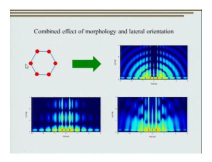
So if I have a hexagonal arrangement of my spherical patterns well I do get a pattern which correspond it to my spherical form factor right leg which we had derived over here so here we have a spherical form factor but the way it is arranged the lattice is hexagonal so therefore there is a superposition of these two things and we do get a very different pattern right.
