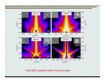
So here again I have chosen one particular example and try to show you how exactly we can see in situ growth of particles so here again we are having the growth of germanium on silicon 001 substrate right so here you see that as the sample or as the quantum dot is growing we do see that there is a change in the scattering pattern and also all these things can be confirmed by doing say AFM or scanning electron microscopy.
