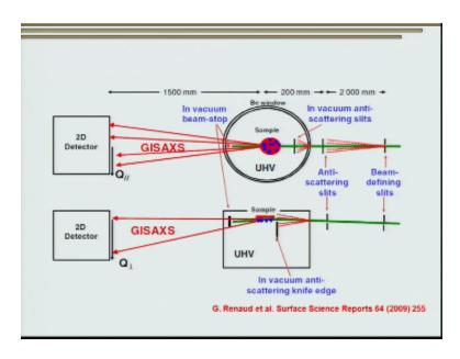
So this shows another the same thing in a different assembly again note the distance the distance between your sample and the detector is huge and there is a there should be a beryllium window over here so that your X rays can pass and here you see that is almost normal you see how small the angle is ray and you see here you get all the information in plane information over here straight away on your 2D detector while out of plane information is over here to perpendicular right.
