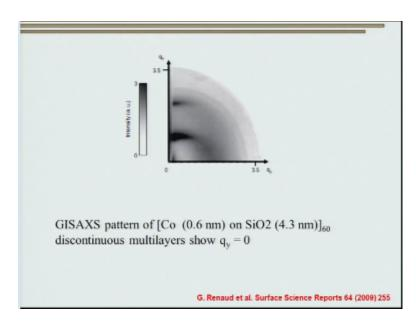
So cheat or rather experimental result of GISAXS pattern of the cobalt 0.6 nanometer on silica 4.3 nanometer 60 such layers discontinuous multi-layer shows which you see it shows qy = 0 here is qy but you see your qs it you see nice Bragg diffraction peaks corresponding to cobalt so you can imagine that how you can use so I am not showing the analysis part over here but using this you see this is in the reciprocal space.
