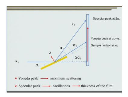
I will talk about in details in the next slide but what I want to want you to remember is that the specular as well as the Yoneda peak okay which occur which show diffraction in the Z Direction gives you a lot of information about in a direction perpendicular to the substrate of the film okay.
