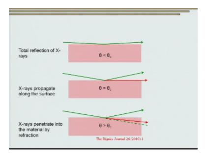
And obtain a lot of information which is pertaining to within the surface or normal to the surface or subsurface in grazing incidence geometry now this particular point is exploited extensively while doing grazing incidence small-angle x-ray scattering.
