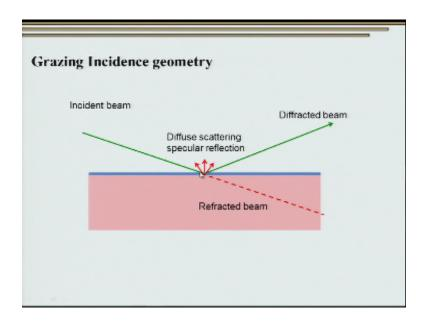
Wherein we not only have a substrate but also we have a thin film or say something like a quantum dots different morphology or say nano particles which are deposited on the surface of this substrate so you can imagine that by choosing a proper combination or rather a proper value of  $\theta$  we can get different conditions.
