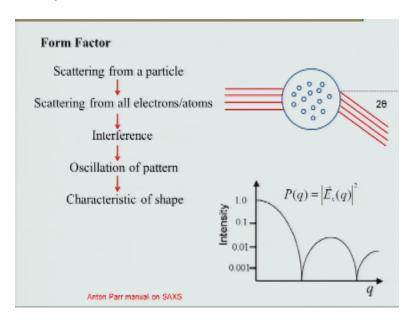
So as we were moving let us consider and a particle and the x-ray is getting scattered from the particle, we know that there is going to be scattering from all the electrons and therefore all the atoms. Now these views the scattered waves are going to interfere with each other and this oscillation pattern is going to have a characteristic shape. Here again I have shown you the variation of intensity as a function of Q which is nothing but the reciprocal vector.
