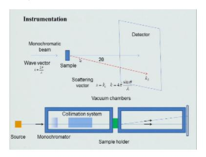
Once this wave with a wave vector of  $2\pi$  by  $\lambda$  passes through the sample it gets scattered and we have to place a detector at a far distance the far distance is at a very large distance the large distance, I hope you remember is required because the angle associated with it is very small so in order to see an appreciable difference and to distinguish between the incident and the diffracted beam we have to keep the detector at a much larger angle.
