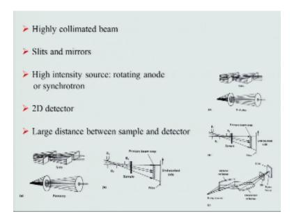
So I hope you appreciate that we need a highly collimated beam which can be obtained using slits and mirrors and this high intensity source consists of rotating anode or a synchrotron, till date the small-angle x-ray scattering carried out using synchrotrons is probably yielding much deeper insights into the understanding of various materials than a laboratory-scale small-angle x-ray scattering.
