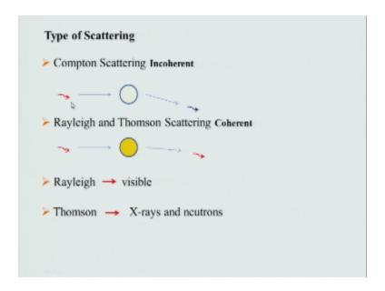
So we have an x-ray photon which interacts with an electron and you do get another x-ray photon which has different frequency, rather a lower frequency and therefore a lower energy than the incident x-ray photon. Therefore this entire process is incoherent that is the energy is not conserved and this corresponds to an elastic scattering. However there is also what is known as relay or Thomson scattering which essentially is elastic and coherent.
