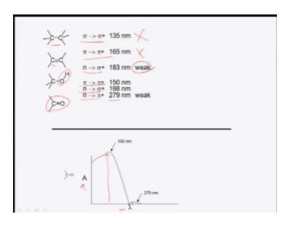
And I can actually go and tell different terms of this is saturated carbon bonds where we can see that is the only possible thing is  $\sigma$  to  $\sigma$ \* is very high energy not possible in visible spectroscopy CC single bond  $\pi$  to  $\pi$ \* is also not possible. And the end to  $\sigma$ \* in this case very weak, so may be possible 183 and then you can have group that is the alcohol, you can have  $\sigma$  2  $\pi$  to  $\pi$ \* x  $\sigma$ \* into  $\pi$ \* transition.
