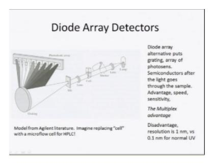
Normally and this is extended way of diode array and I am showing you this are the 328 diodes which are slit at the sample radiation comes under the sample it is detective diode well so that's all in the next class we will I will show you some more spectrum from the UV visible results in my lab and some of the details things which I gathered from literature and then we move on to the next techniques.
