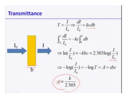
And this can be even formulated by this way suppose I is the initial radiation initial intensity of the radiation and this is the path length and I is the final which is coming out I/I0 d I/d0 is basically Kc db you can say this k is the constant and then one can get this kind of formula and the  $\varepsilon$  which is the molecular absorptivity can be written by k / 2.303 which is from log.
