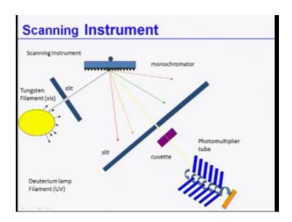
Now in scanning instrument we do not do that what I do is that we have to tungsten filaments are visible and even day to lamp that is deuterium lamp for UV this is d20 okay this is tungsten as showed so both of them actually comes and process through the slit and then you have a monochromatic here how the mono-chromator works is basically as crystals.
