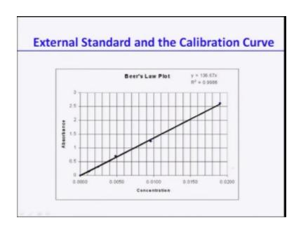
Then one can actually use this external standard and calibrate this curve so this is the absorption and this is the concentration you can see it the follow of the linear raw law where r is very high so the fitting which is almost 99%.
