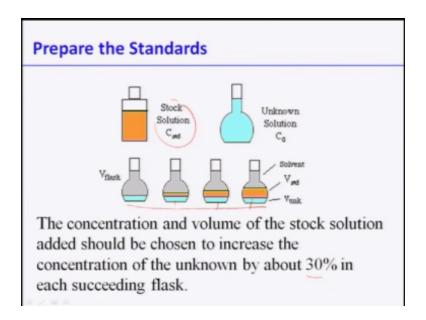
How do you prepare the standards can be prepared in different ways like this is stock solution and then you can dilute it and get the different concentrations and that is why you can prepare the standards. The concentration and volume of the stock solutions added should be chosen to increase the concentration of the unknown by about 30% in each flask. That is this is the known and this is the unknown so you add unknown quantity concentrations and then add up to maximum 30%.
