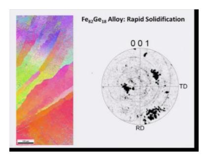
Now as for this texture is cancer which are just now I mentioned if I just use this end put a plot inverse pole figure from the gain map you can see there is fibrous texture paste and you can see this kind of nature of this texture clearly present on 11 orientations in a typical ID wealth and TD plot and there are obviously orientations of the grains which are predominantly patient in along these directions ,so one can actually obtain exactly the nature of texture from this analysis.
