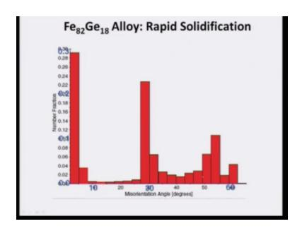
And if we do this again this from the same grain if we if I plot the grain boundary number of fractional gain boundary submission triangle again we see large number of gains of the base small mis-orientation less than about 7.5 degrees and they are actually having small angle boundaries what are there are grains which having large angle gain motives so gain bound the information be easily obtained.
