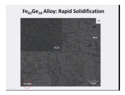
If we under cumulative n little deeply 140 k I am just showing the optical micrograph can see the big grains here again and within the big gain there are so many small gains patients similar nature which have shown just one slide before and if we zoom out the picture you can see the segregation of genetic pattern inside the grains actually if you are under cool it even much higher level by 190 k.
