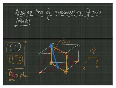
So, redoing line of intersection of two planes. Let us take up exactly the same problem, so this is one of the things another geometric application of Weiss zone law. Two applications of Weiss zone law, if two planes are given, you can find the common direction, if two directions are given you can find the plane passing through the direction.
