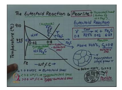
A Gamma phase of 0.8 weight percent carbon, at 725 degrees Celsius on further cooling will form Alpha plus F e 3 C and that was our Pearlite; this was the Pearlite. So, which means in this case, we now have lots of Alpha which have already formed in the Gamma plus Alpha phase field. But the remaining Gamma whatever is there at 725 degrees Celsius is of the right composition 0.8 weight percent carbon and at right temperature 725 degree Celsius for the eutectoid reaction to happen.
