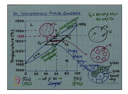
So, isomorphous system or isomorphous phase diagram is nothing, but what we have been seeing. The copper nickel diagram is an example of an isomorphous phase diagram. All it means that there is a single crystalline phase at lower temperature from all the way from starting from one end copper to another end nickel. Similarly there is a single liquid phase all the way from the copper end to the nickel end at the higher temperature.
