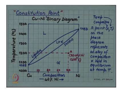
Basically as we have seen that phase diagram and as I told you we will mainly focus on binary diagram, which means two components and in this particular example the two components are copper and nickel, which is written on the x axis here and the temperature is on the y axis. So, our thermodynamic variables a composition the composition and composition in this particular case is being expressed as weight percent nickel.
