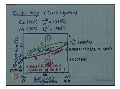
Example; copper nickel copper nickel alloy in phase background jar din or phase background terminology alloys are also sometimes called systems. You can say copper nickel alloy or you can say copper nickel system.
