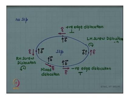
So, let me mark outside region as no slip and inside as the slip. So, this loop also qualifies the definition that is the boundary between a slipped region and an un slipped region. So, the slip is happening now inside the loop and the outside has not slipped. If we have so, this becomes a dislocation line.
