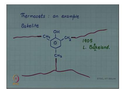
A really interesting example of a thermoset is a Bakelite, you can see in the Bakelite monomer which is shown here this is the aromatic or benzene ring, 3 of the hydrogen's are substituted by CH 2 group and 1 hydrogen is substituted by the OH group and these CH 2 groups then have 1 free bond to connect when other monomers, but since each monomer unlike polyethylene, where each monomer had only 2 free bonds.
