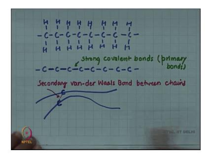
Let us explain, the van-der Waal bonding means, now I was drawing the carbon-carbon chain like this with hydrogen's attached to the carbon this is the structure of polyethylene which we have discussed.
