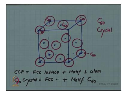
So, if I can now draw an FCC unit cell, you are familiar with FCC unit cell. So, we begin with a cube and we place lattice points at each of the corners and at the 6 face centers. So, all these little crosses are lattice points and if I now think in terms of the C 60 solid or a C 60 crystal. So, I place the C 60 molecule; the truncated icosahedron molecule at each of the lattice points.
