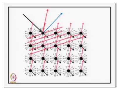
So, let us try that. So, I remove the blue planes now and draw a new set of planes the red plane from which again the incident beam and the red diffracted beam make equal angles.
