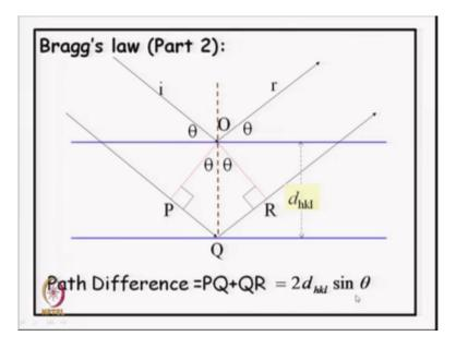
So, we take up this proof here. So, the blue line shows the first the top crystal plane which is receiving the incomingX Ray eye and is reflecting it or diffracting it in the direction r the incident angle theta is equal to the reflection angle theta let us introduce now the second plane at a distance dhkl.
