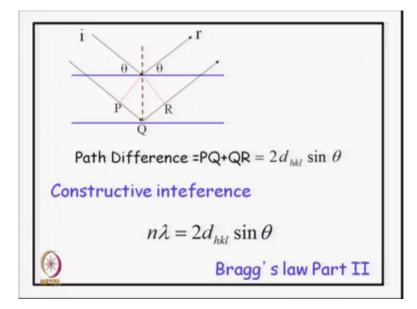
So, for constructive interference path difference should be an integral multiple of the wavelength. So, this is what gives you in the final Bragg's law that the path difference is integral multiple times the wavelength and lambda is equal to 2 dhkl sin theta. This completes our derivation and description of Bragg's law.
