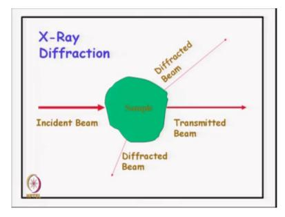
So, let us look at X-Ray diffraction, we have an incident beam we falling on a sample we expect a transmitted beam which is in the same direction as the incident beam. If all of the X-Rays is not absorbed there will be a transmitted beam this is what is used in normal medical use of X-Rays when you when we have X-Ray photographs, but if the sample is crystalline then you can expect beams other than the transmitted beam; beams in direction other than the
